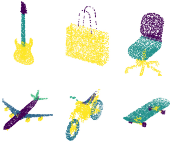
Figure 1: Examples of 3D point clouds of objects from the ShapeNet part-segmentation challenge [23]. The colors of the points represent the part labels.
