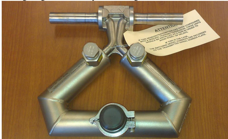
Figure 7: Photograph of the Micromotion CMF025 Coriolis flow meter used in the CMTS Valve Box on all three supply circuits
