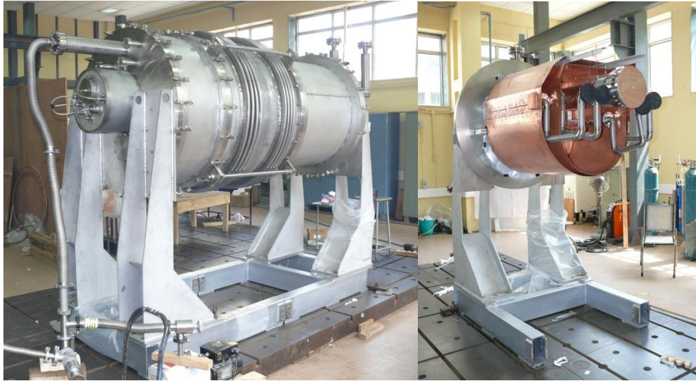
Figure 6: Photographs of the Feedcap and Endcap at during fabrication and testing at BARC
