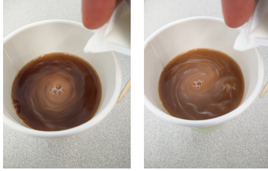
FIGURE 2. Milk mixing into an approximately axisymmetric vortex.
