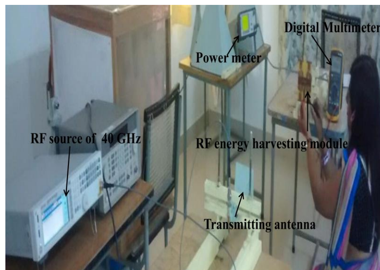
Figure 6. Measurement of output DC voltage from the module with respect to RF input voltage from RF source.
