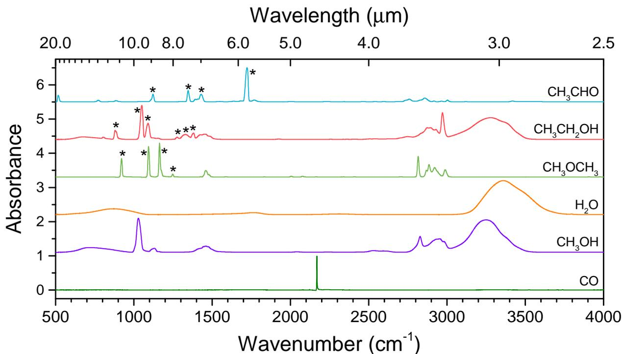
Fig. 1: Spectra of pure acetaldehyde (blue), ethanol (red), dimethyl ether (green), water (orange) methanol (purple), and CO (dark green) normalized to one in the range of 2.5 to 20.0  $\mu\text{m}$ . The bands investigated in this work are indicated with an asterisk (\*).
