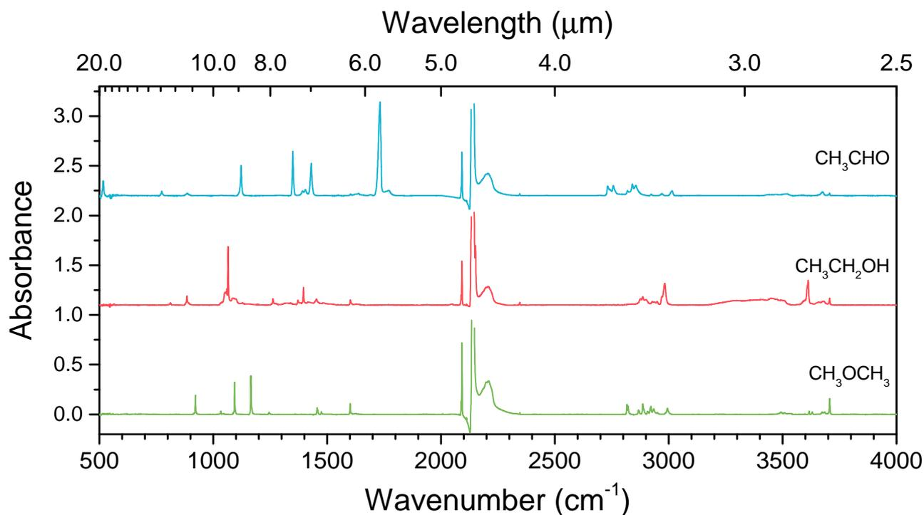
Fig. A.2: Spectra of acetaldehyde (blue), ethanol (red), and dimethyl ether (green) mixed in CO at 15 K in the range of 2.5 to 20.0  $\mu\text{m}$ .
