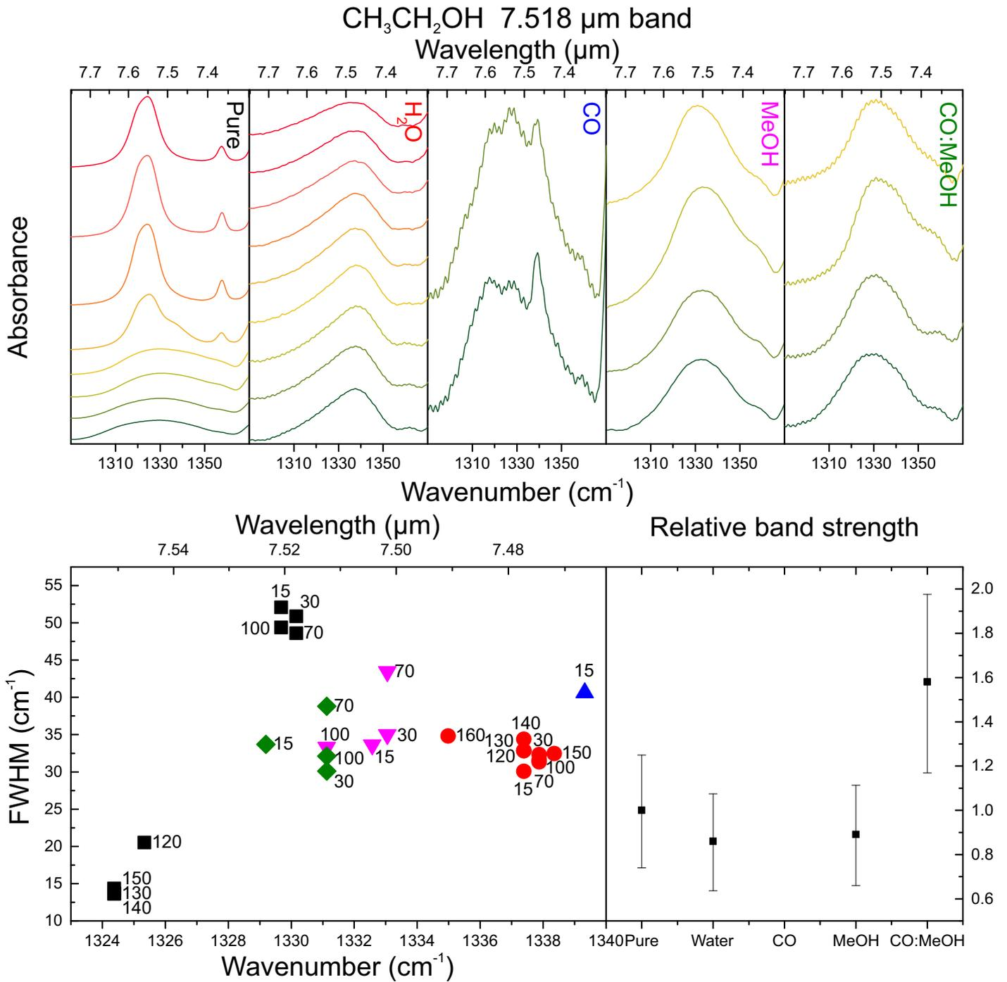
Fig. C.8: Top: from left to right the ethanol 7.518 μm band pure (black) and in water (red), CO (blue), methanol (purple), and CO:CH<sub>3</sub>OH (green) at various temperatures. Bottom left: peak position vs. FWHM plot, using the same colour coding. Bottom right: the relative band strength for the 7.518 μm band at 15 K in various matrices.
