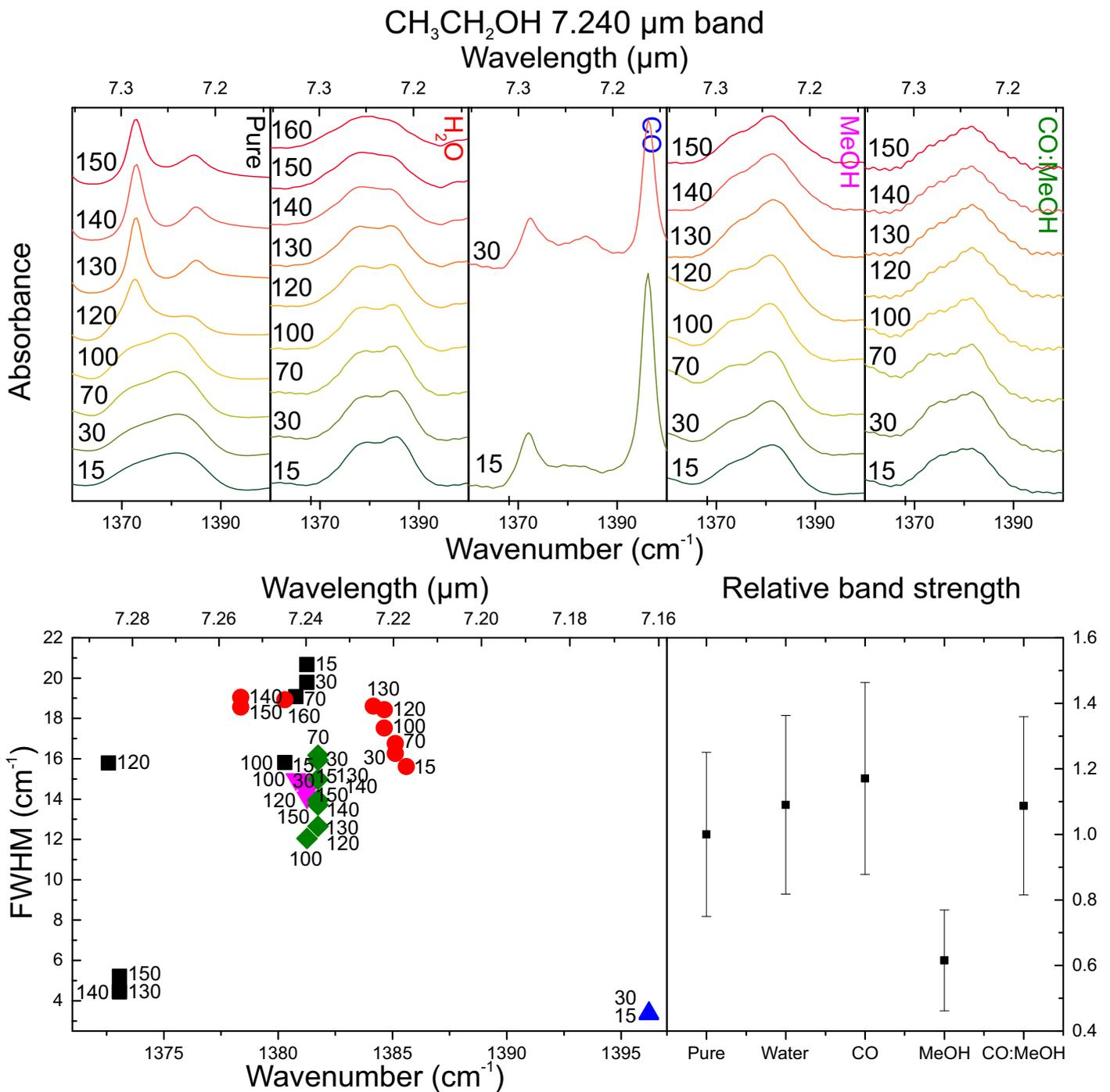
Fig. 3: Top: from left to right the ethanol 7.240 μm band pure (black) and in water (red), CO (blue), methanol (purple), and CO:CH<sub>3</sub>OH (green) at various temperatures. Bottom left: peak position vs. FWHM plot, using the same colour coding. Bottom right: the relative band strength for the 7.240 μm band at 15 K in various matrices.
