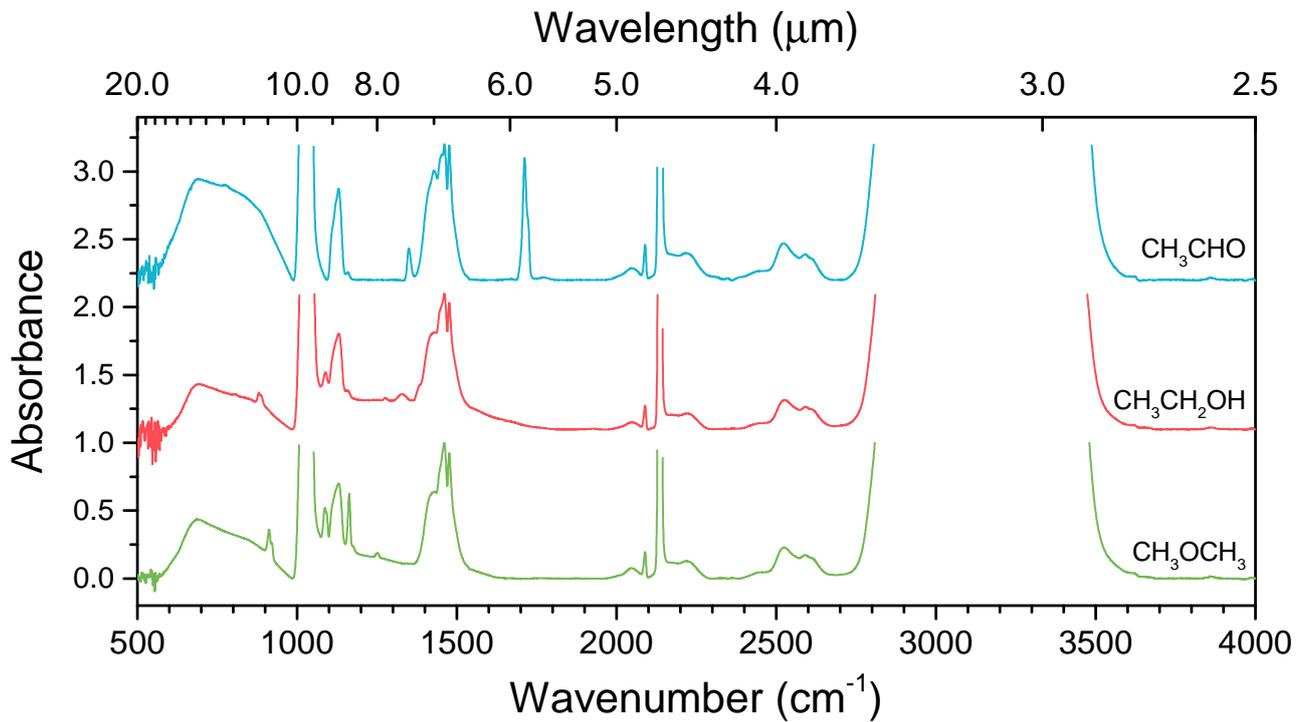
Fig. A.4: Spectra of acetaldehyde (blue), ethanol (red), and dimethyl ether (green) mixed in CO:CH<sub>3</sub>OH at 15 K in the range of 2.5 to 20.0  $\mu\text{m}$ .
