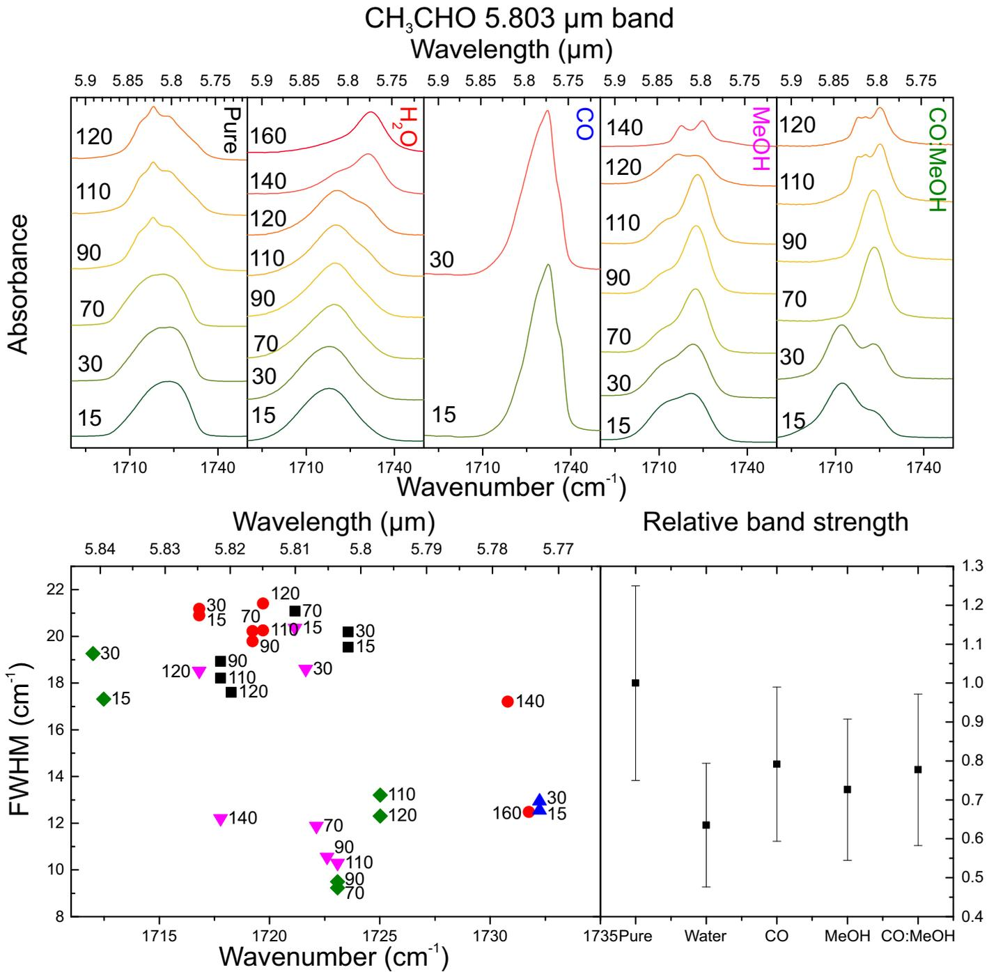
Fig. C.3: Top: from left to right the acetaldehyde 5.803  $\mu$ m band pure (black) and in water (red), CO (blue), methanol (purple), and CO:CH<sub>3</sub>OH (green) at various temperatures. Bottom left: peak position vs. FWHM plot, using the same colour coding. Bottom right: the relative band strength for the 5.803  $\mu$ m band at 15 K in various matrices.
