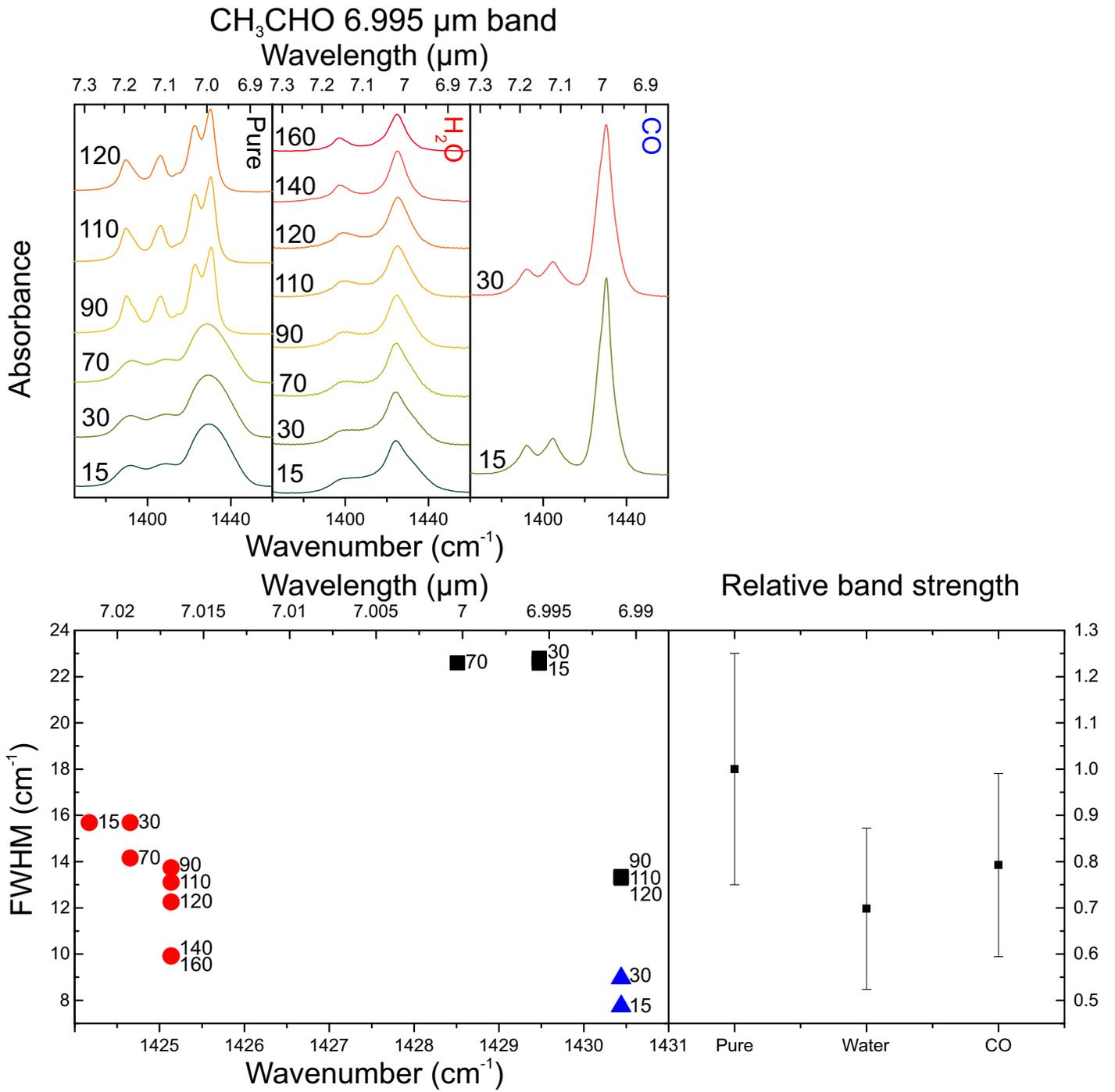
Fig. C.2: Top: from left to right the acetaldehyde 6.995  $\mu$ m band pure (black) and in water (red) and CO (blue) at various temperatures. Bottom left: peak position vs. FWHM plot, using the same colour coding. Bottom right: the relative band strength for the 6.995  $\mu$ m band at 15 K in various matrices.
