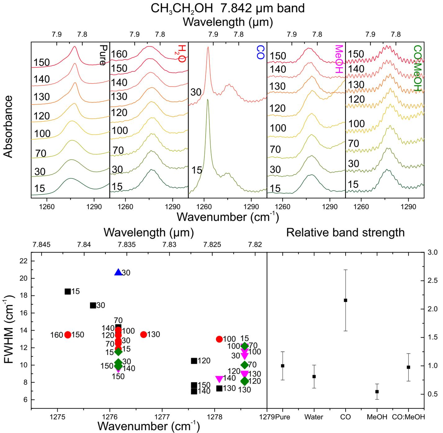
Fig. C.7: Top: from left to right the ethanol 7.842 μm band pure (black) and in water (red), CO (blue), methanol (purple), and CO:CH<sub>3</sub>OH (green) at various temperatures. Bottom left: peak position vs. FWHM plot, using the same colour coding. Bottom right: the relative band strength for the 7.842 μm band at 15 K in various matrices.
