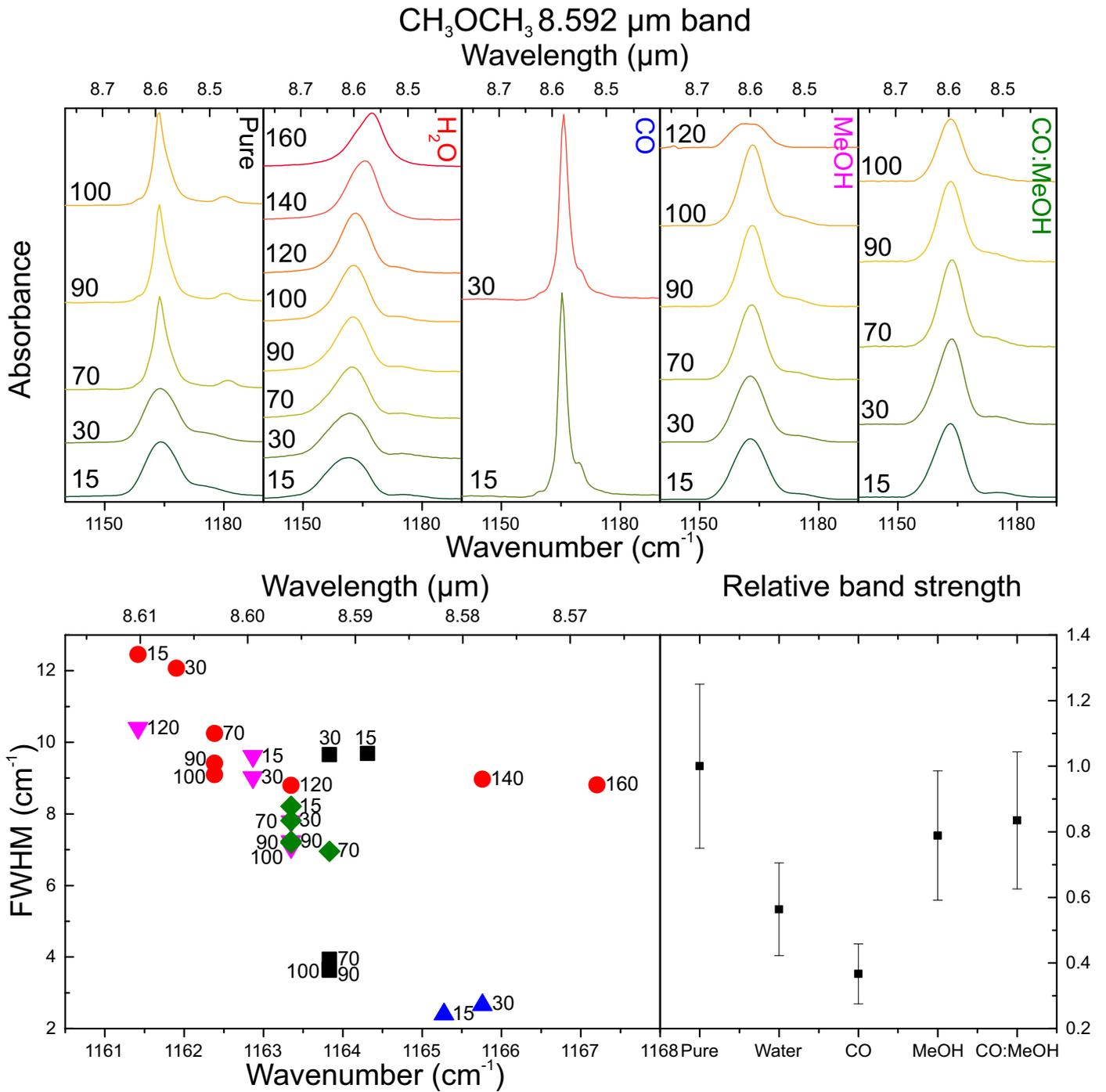
Fig. C.11: Top: from left to right the dimethyl ether 8.592 μm band pure (black) and in water (red), CO (blue), methanol (purple), and CO:CH<sub>3</sub>OH (green) at various temperatures. Bottom left: peak position vs. FWHM plot, using the same colour coding. Bottom right: the relative band strength for the 8.592 μm band at 15 K in various matrices.
