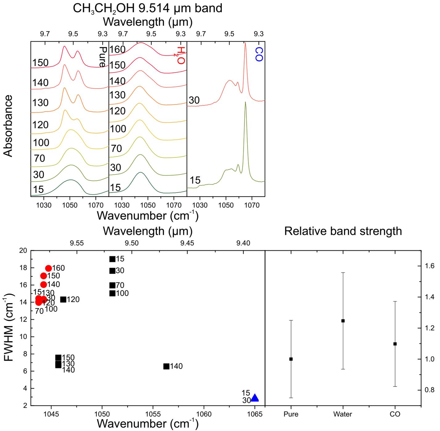
Fig. C.5: Top: from left to right the ethanol 9.514  $\mu$ m band pure (black) and in water (red) and CO (blue) at various temperatures. Bottom left: peak position vs. FWHM plot, using the same colour coding. Bottom right: the relative band strength for the 9.514  $\mu$ m band at 15 K in various matrices.
