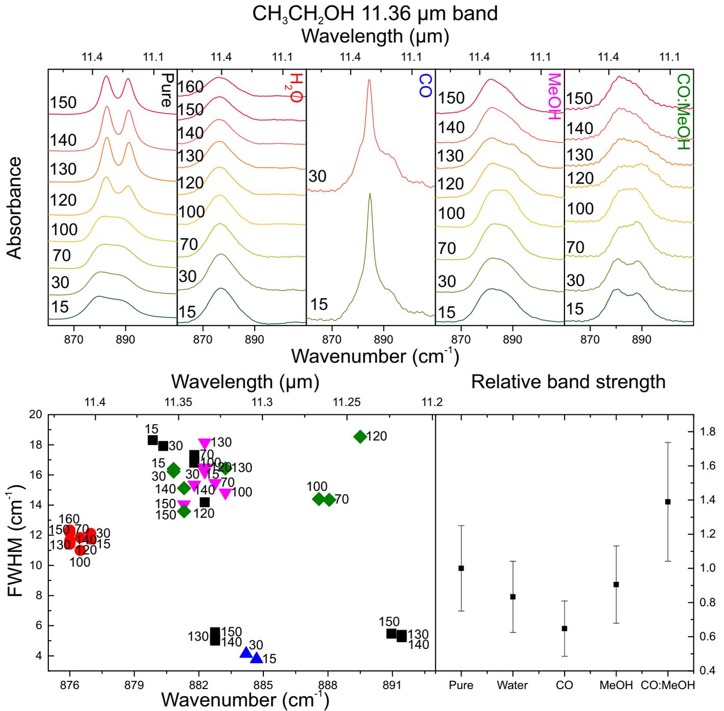
Fig. C.4: Top: from left to right the ethanol 11.36  $\mu$ m band pure (black) and in water (red), CO (blue), methanol (purple), and CO:CH<sub>3</sub>OH (green) at various temperatures. Bottom left: peak position vs. FWHM plot, using the same colour coding. Bottom right: the relative band strength for the 11.36  $\mu$ m band at 15 K in various matrices.
