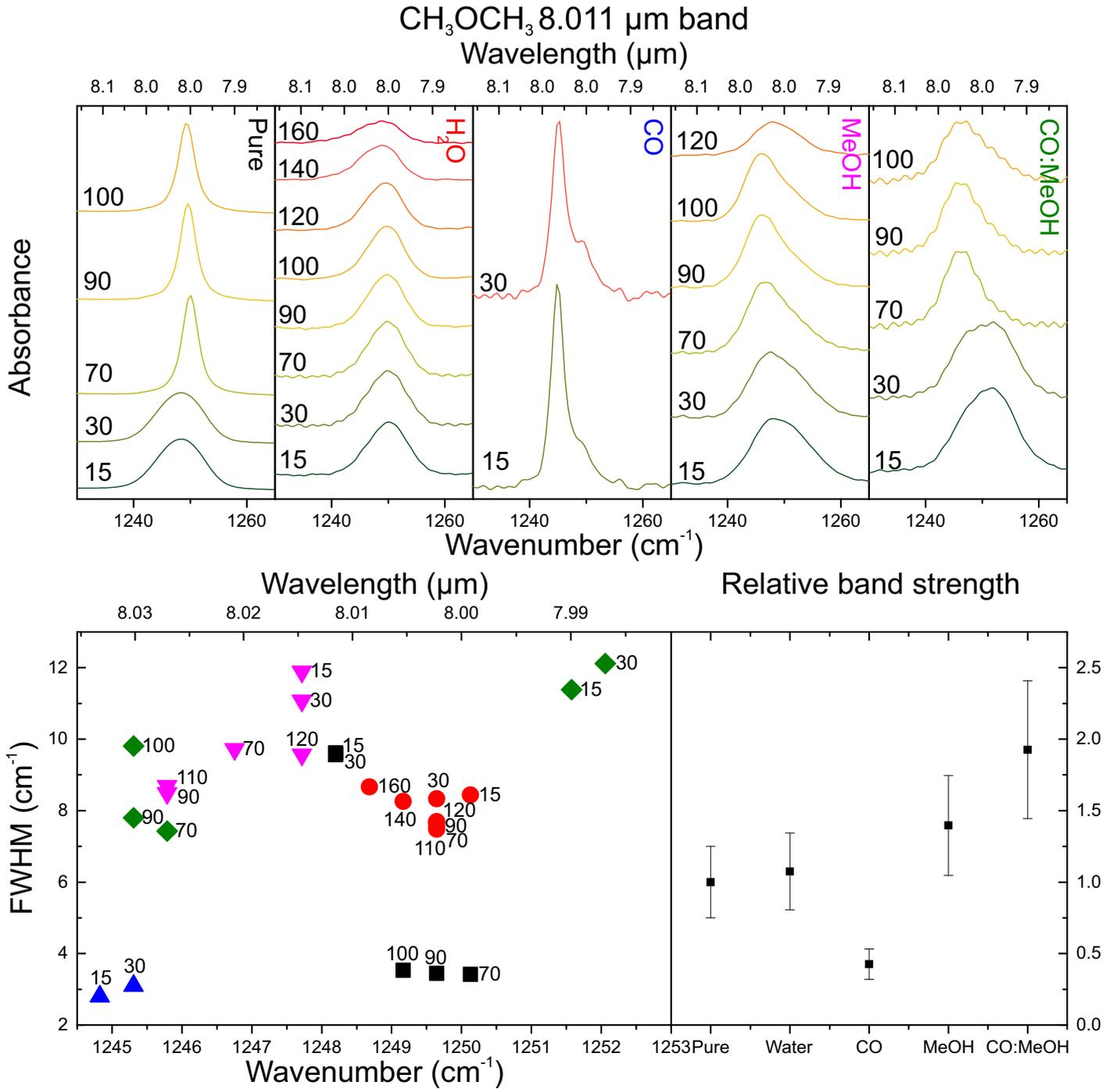
Fig. 4: Top: from left to right the dimethyl ether 8.011  $\mu$ m band pure (black) and in water (red), CO (blue), methanol (purple), and CO:CH<sub>3</sub>OH (green) at various temperatures. Bottom left: peak position vs. FWHM plot, using the same colour coding. Bottom right: the relative band strength for the 8.011  $\mu$ m band at 15 K in various matrices.
