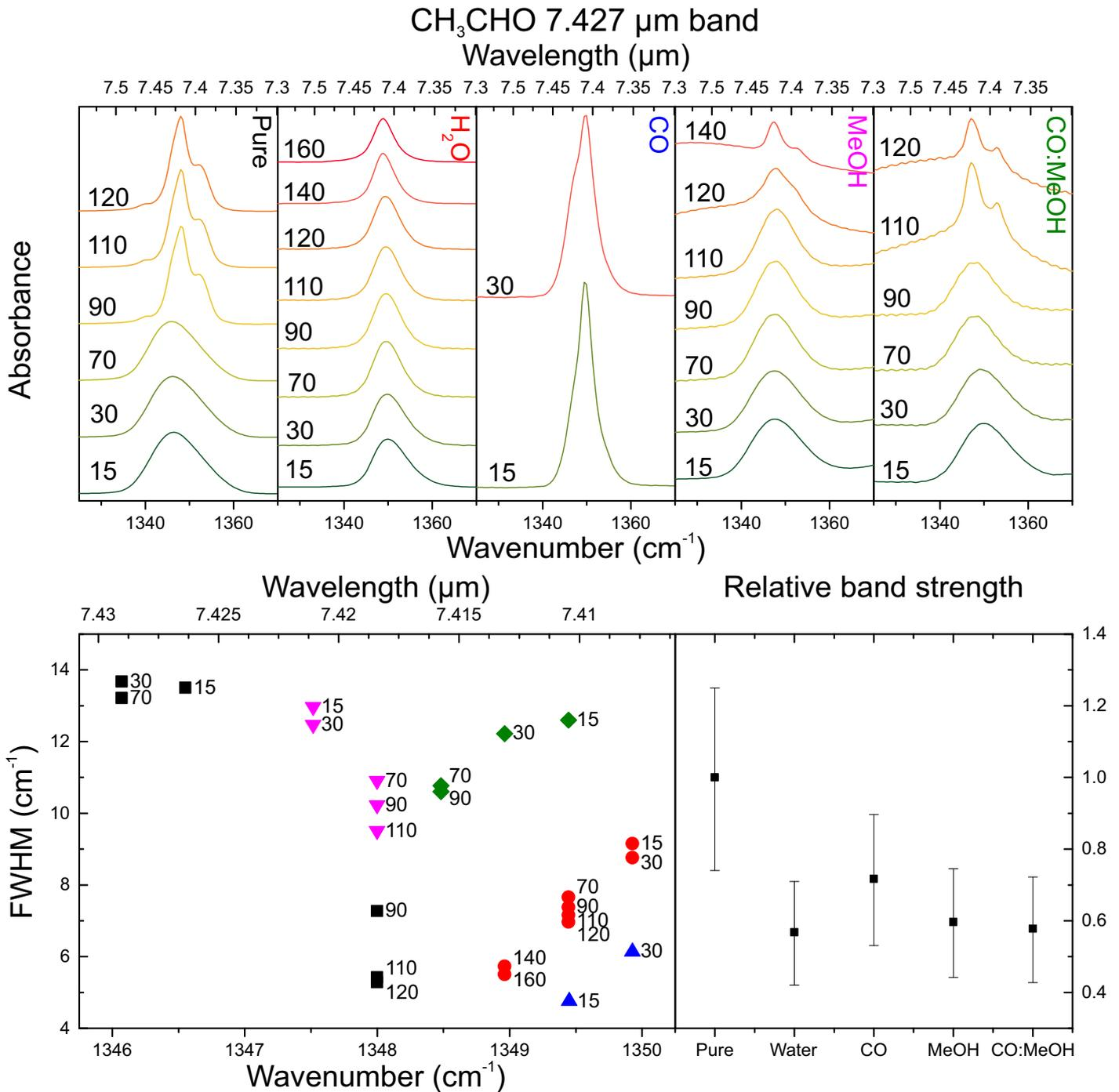
Fig. 2: Top: from left to right the acetaldehyde 7.427  $\mu\text{m}$  band pure (black) and in water (red), CO (blue), methanol (purple), and CO:CH<sub>3</sub>OH (green) at various temperatures. Bottom left: peak position vs. FWHM plot, using the same colour coding. Bottom right: the relative band strength for the 7.427  $\mu\text{m}$  band at 15 K in various matrices.
