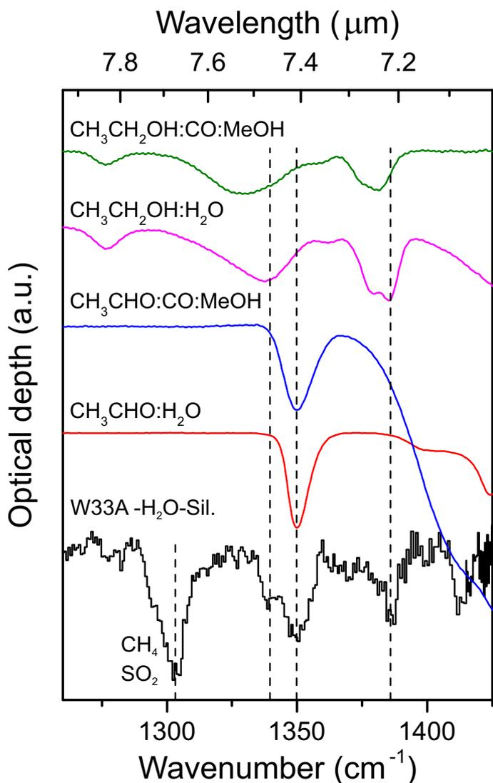
Fig. 5: Continuum and water and silicate subtracted spectrum of W33A plotted together with ice spectra of ethanol and acetaldehyde at 15 K, mixed in CO:CH<sub>3</sub>OH and H<sub>2</sub>O. Features in the W33A spectrum are indicated with dashed lines at 7.22, 7.40, and 7.47  $\mu\text{m}$ . The large spectral feature at 7.67  $\mu\text{m}$  is due to CH<sub>4</sub> and SO<sub>2</sub>.
