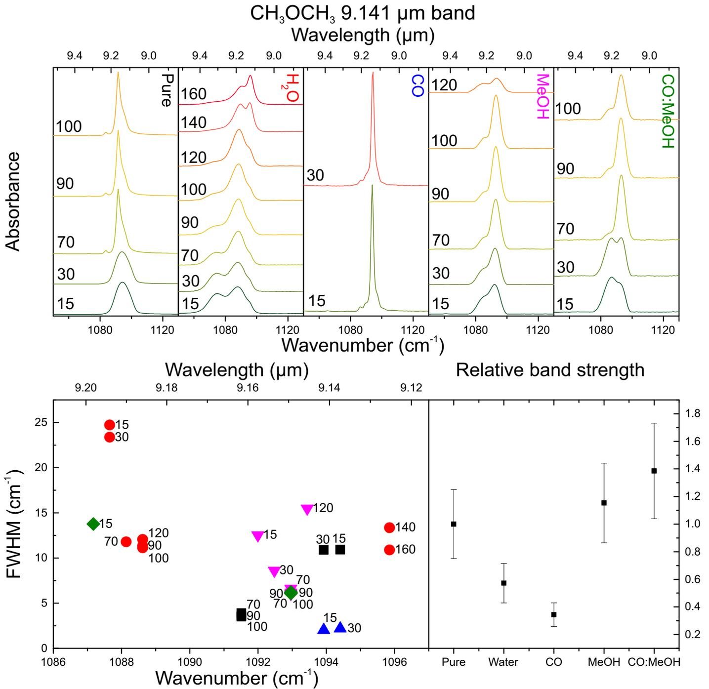
Fig. C.10: Top: from left to right the dimethyl ether 9.141  $\mu$ m band pure (black) and in water (red), CO (blue), methanol (purple), and CO:CH<sub>3</sub>OH (green) at various temperatures. Bottom left: peak position vs. FWHM plot, using the same colour coding. Bottom right: the relative band strength for the 9.141  $\mu$ m band at 15 K in various matrices.
