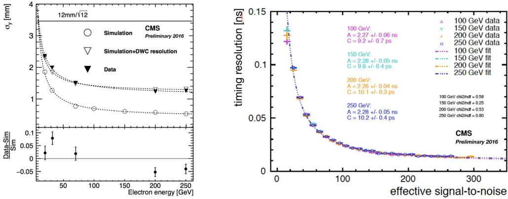
**Figure 2.** Left: Spatial precision as a function of electron energy at  $6X_0$  depth. Right: Intrinsic timing resolution for time differences within a cluster for different electron energies as a function of  $(S/N)_{\text{eff}}$ .
