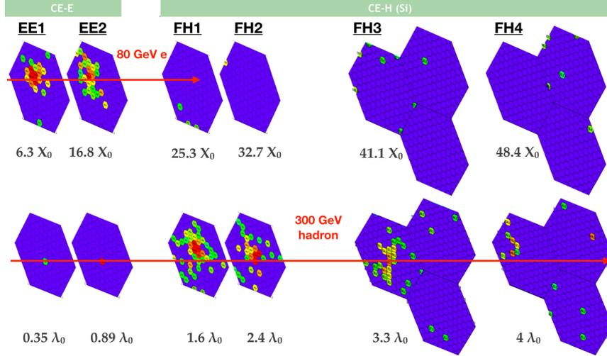
**Figure 3.** Event display for the silicon-based prototype for 80 GeV electrons (top) and 300 GeV hadrons (bottom) for the July 2017 beam test. The AHCAL is not shown.
