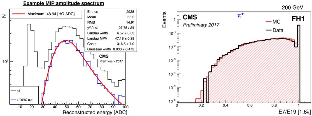
**Figure 4.** Left: Amplitude spectra for one cell induced by 150 GeV muons. Right: Transverse shower shape for 200 GeV pions in the first layer of the hadronic section.
