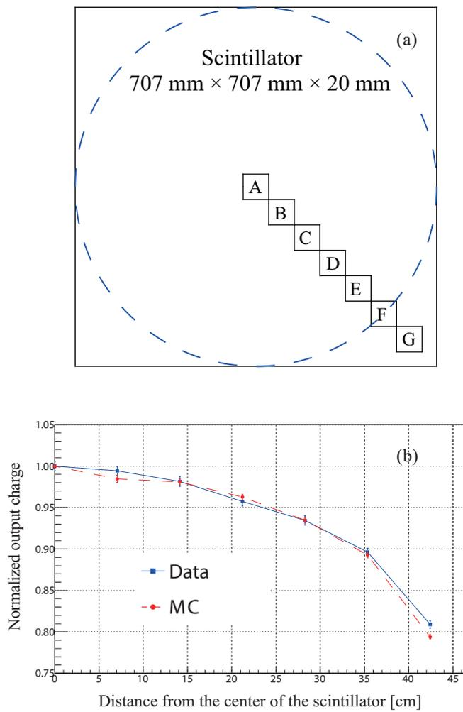
**Figure 8.** (a) Experimental set-up for the uniformity measurement. (b) Uniformity of the prototype detector (with reference to the center of the scintillator).
