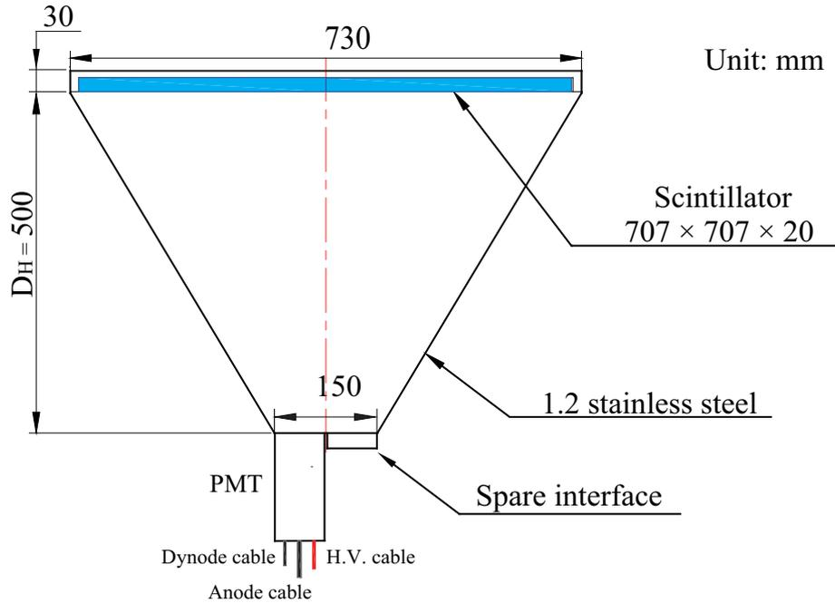
**Figure 1.** Schematic diagram of the prototype scintillator detector.
