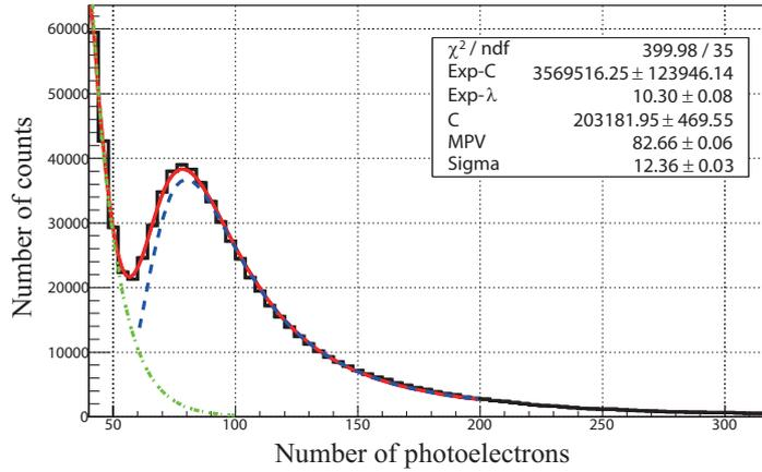
**Figure 6.** Single-particle distribution of the prototype detector. The fitted plots include detector noise (dashed-dotted line), signal of a single particle (dashed line), and their sum (solid line).
