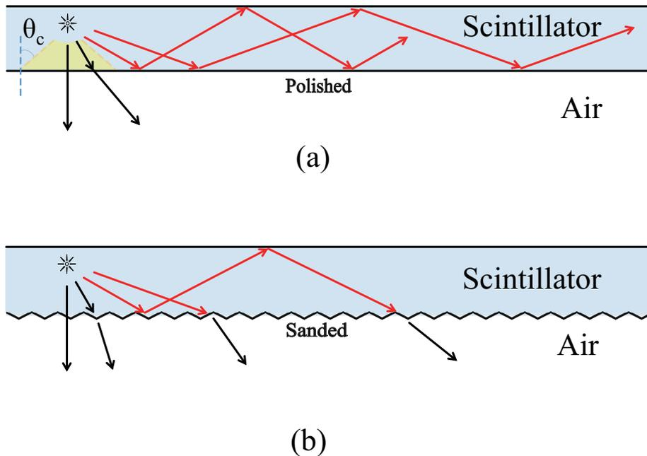
**Figure 2.** Refraction and total internal reflection of light at the interface between the scintillator and the air light guide. (a) Two polished surfaces; (b) One surface polished and one surface sanded.
