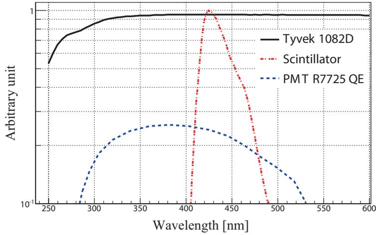
**Figure 4.** Emission spectrum, quantum efficiency, and Tyvek 1082D reflectivity used in the Optical Model.
