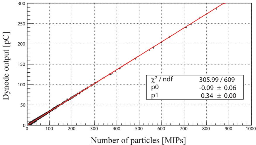
**Figure 9.** Linearity of the prototype detector.
