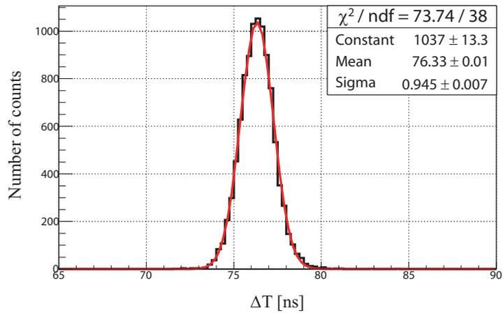
**Figure 7.** Time resolution of the prototype detector.
