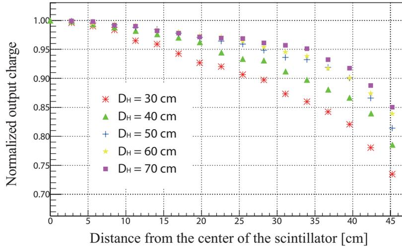
**Figure 5.** Simulated uniformity (with reference to the center of the scintillator) at different  $D_H$ .
