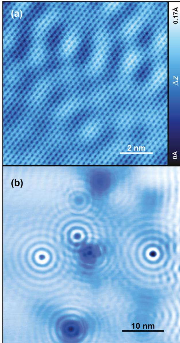
Figure 8. Qualitative proof of the instrument performance at base temperature  $T_{MC} = 29$  mK. (a) Atomic resolution of Cu(111) on a 10 nm x 10 nm area ( $I_t = 10$  nA,  $V_S = 12$  mV). (b) Measured quasi-particle interference (QPI) on the Cu(111) surface ( $I_t = 200$  pA,  $V_S = 100$  mV). The measurements were done with a PtIr tip.
