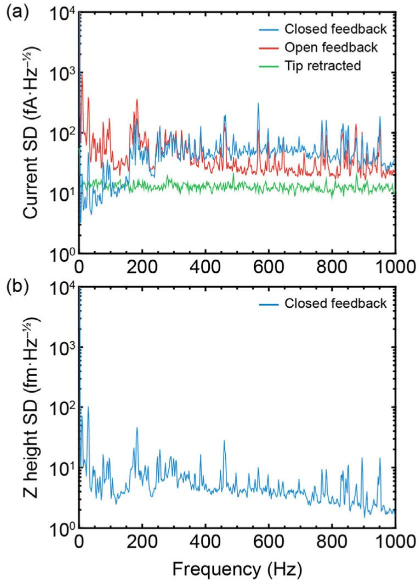
Figure 7. (a) Measured spectral density of the current signal for frequencies up to 1 kHz. Shown is the open (red) and closed (blue) feedback noise compared to the situation of a retracted tip (green), i.e. out of tunneling range ( $I_t = 500$  pA,  $V_s = 10$  mV,  $T_{MC} = 43$  mK). The data were taken with a PtIr tip on a thick Pb film grown on W(110). (b) Measured spectral density for the z-signal under the same measuring conditions.
