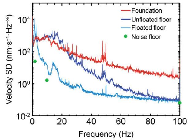
Figure 2. Vibrational noise measurements of the lab, measured on the foundation (red), on the unfloated (dark blue) and floated concrete block (bright blue), respectively. Shown is the velocity spectral density. In addition, the noise floor (green dots) of the used accelerometer in combination with the spectrum analyzer is shown.
