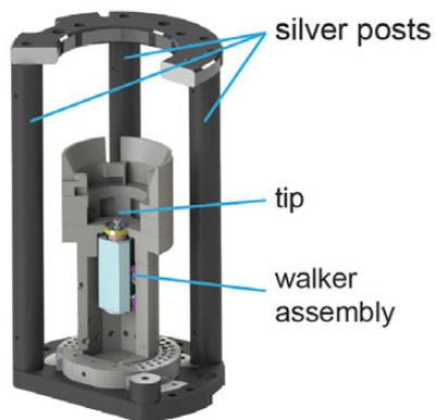
Figure 6. Cut view of the STM body and the silver posts that connect the microscope to the mixing chamber. The tip pointing upward can be moved by the piezo-driven stepper motor, utilizing the Pan design, towards the sample (latter not shown here).
