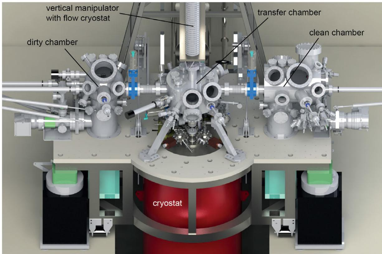
Figure 3. The UHV system comprises three interconnected chambers, separable by valves. The cryostat (red) is below the central vessel. The two satellite chambers are utilized for MBE and CVD preparation, as well as sputtering and annealing of samples.
