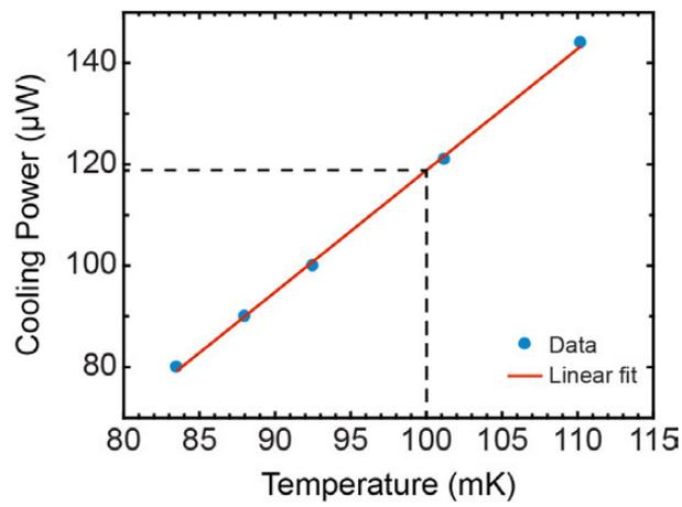
Figure 5. Cooling power of the JDR-50 dilution refrigerator as a function of the temperature measured at the mixing chamber without the microscope attached. At 100 mK the cooling power is 115  $\mu\text{W}$  with a continuously running JT-compressor.
