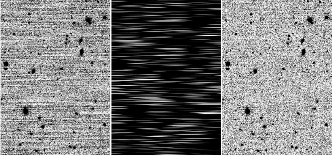
Fig. 3.—: Removal of pattern noise in MzLS data. Left: raw image; middle: noise pattern constructed by a low-pass filter; right: image after pattern removal.
