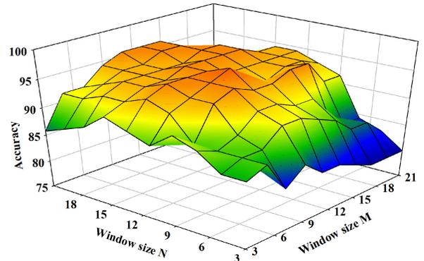
Fig. 4. Graph shows the accuracy rates obtained for different normalization and feature detection window sizes ranging from  $M=N=3$  to 21 for one trial of leave-one-out cross-validation method.
