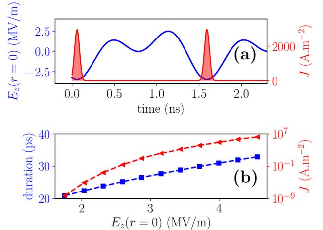
Figure 1: Axial electric field applied on the cathode (blue trace) and the emitted current density (red shaded curve) (a). Evolution of the current density peak value (squares) and rms electron pulse duration (triangles) as function of the applied peak field (b). The peak-field configuration and associated parameters are detailed in Sec. 2. Note that these are ideal numbers calculated at the cathode surface without accounting for possible saturation effects of the emission process.
