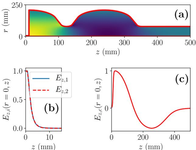
Figure 2: Geometry of the SRF cavity (red trace) with field distribution  $E_z(r, z)$  (a), axial fundamental  $E_{z,1}(r = 0, z)$  and harmonic  $E_{z,2}(r = 0, z)$  electric fields in the vicinity of the cathode surface and axial field  $E_{z,c}(r = 0, z)$  along the 1+1/2-cell cavity (c). All the field are normalized to their peak amplitudes.
