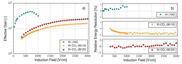
Figure 4: Effective gain (a) and relative energy resolution (b) as a function of the induction field for pure krypton,  $Kr-CO_2$  (90:10) and  $Kr-CO_2$  (80:20). The energy resolution is relative to the first data point taken.
