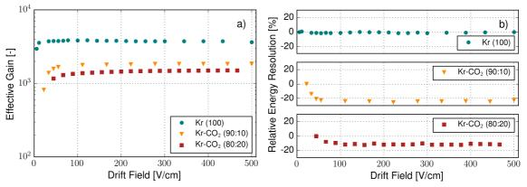
Figure 2: Effective charge gain (a) and relative energy resolution (b) as a function of the electric field in the drift region, for the gas mixtures studied in this work. The energy resolution is relative to the first data point taken.
