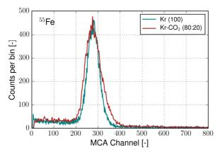
Figure 6: Pulse height distribution recorded for pure krypton and the  $Kr-CO_2(80:20)$  mixture. Energy resolutions measured in pure krypton and  $Kr-CO_2(80:20)$  were, respectively, 22 and 27% (FWHM, 5.9 keV).
