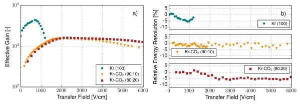
Figure 3: Effective gain (a) and relative energy resolution (b) as a function of the transfer field for pure krypton, krypton- $CO_2$  (90:10) and krypton- $CO_2$  (80:20). The energy resolution is relative to the first data point taken.
