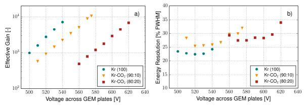
Figure 5: Charge multiplication, (a) and energy resolution, b) for the GEM foils operated in different Kr-CO<sub>2</sub> mixtures. The electric fields in the drift, transfer and induction regions were for each mixture, respectively (V×cm<sup>-1</sup>): pure krypton (200/650/580), Kr-CO<sub>2</sub>(90:10) (333/1930/2500), Kr-CO<sub>2</sub>(80:20) (310/2800/1500).
