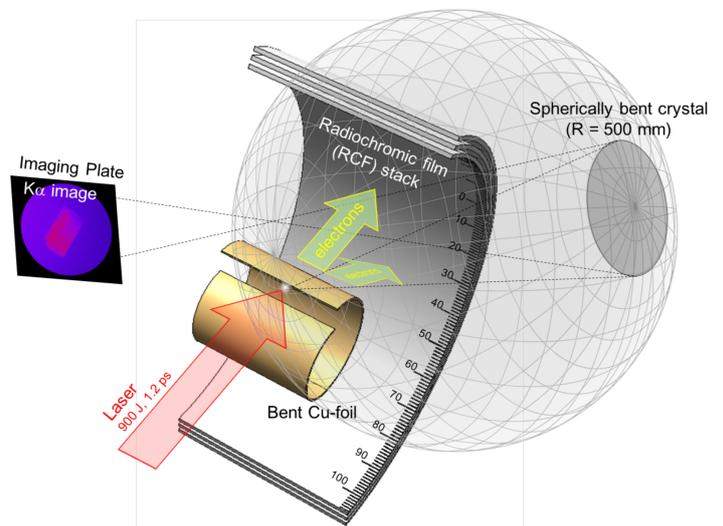
A schematic sketch of the experimental setup. The main laser pulse, containing three equal beams of LFEX laser, enters the slit at grazing direction. The target is made from copper, to allow the Cu-K $\alpha$  imaging of the hot electron with the use of a spherically bent crystal, shown behind the target. Also, a curved large-angle radiochromic film (RCF) stack, is placed around the target.
