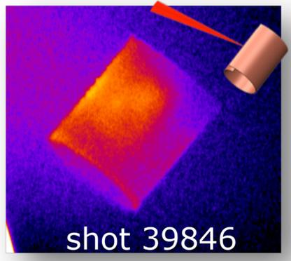
Image obtained by Cu-Ka emission from a snail target, irradiated by only the main laser pulse, which contained three LFEX beams, focused on the target surface through the entrance slit. The geometry of view is shown in the inset. The extended signal indicates a guiding of the laser beam inside the target. Assymetry between left and right edges of the target relates to laser alignment issues.
