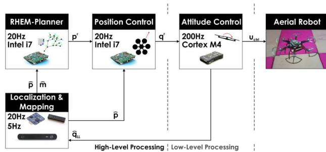
Fig. 7. Overview of the key robot functionalities.
