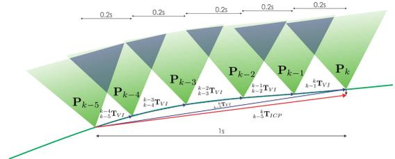
Fig. 8. Point clouds derived at 5Hz are merged in their neighborhood and used altogether for the estimation of the ICP transformation of the robot motion at 1Hz.
