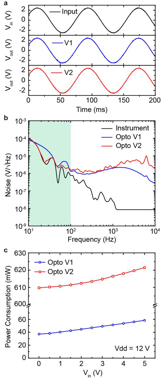
FIG. 3. **Performance of the optocoupler circuits.** **a**, Input versus output signal for the low-power (V1) and low-noise (V2) versions. **b**, Noise as a function of frequency for the two versions compared to the intrinsic noise of the measuring lock-in amplifier. The low-frequency region is highlighted in green. **c**, Power consumption as a function of input voltage (peak-to-peak) for the two versions of the optocoupler circuit.
