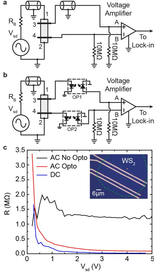
FIG. 5. **Characterization of a  $\text{WS}_2$  field-effect transistor.** **a**, Electrical circuit configuration for local 4-probe AC measurement of a field-effect transistor (FET). **b**, Floating-probe arrangement of the same FET measurement in panel **a**, coaxial cables are omitted for clarity. **c**, Resistance as a function of bias of a  $\text{WS}_2$ -based (FET), measured in the two AC configurations shown in panels **a** and **b** and in DC.
