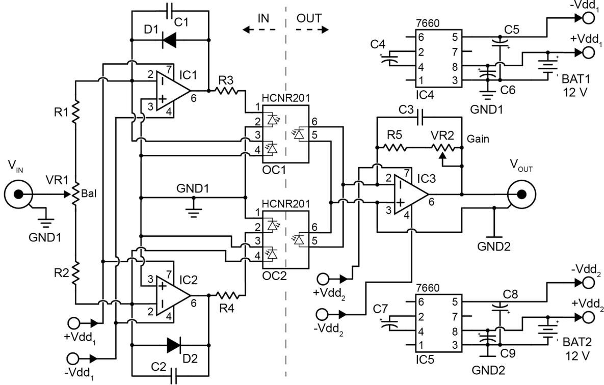
FIG. 1. **Electronic schematic of the bipolar optocoupler circuit.** The circuit is designed around two HCNR201 high-linearity optocouplers (OC1, OC2) powered by two 12 V batteries. Two ICL7660 CMOS voltage converters (IC4 and IC5) are used to supply the required dual voltage ( $\pm 12$  V) to the operational amplifiers (IC1, IC2 and IC3). The vertical dashed line indicates the optical coupling point between the input (IN) and the output (OUT) stages of the circuit.
