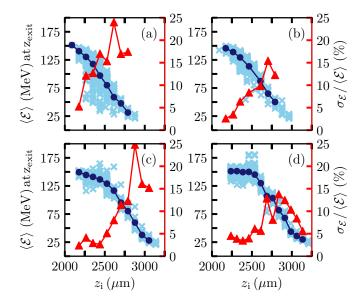
FIGURE 2: Average energy at the exit of the simulation with respect to injected position,  $z_i$  for the  $6^{th}$  electrons, for nitrogen concentration: (a) 2%, (b) 1%, (c) 0.5% and (d) 0.35%. The average of average energy and energy dispersion per slice evaluated along  $z_i$  are represented respectively by the blue dots and the red triangles.
