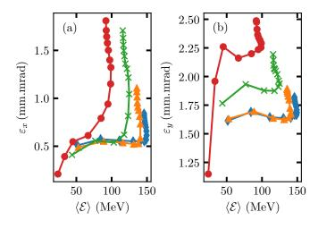
FIGURE 5: Emittance (a)  $\varepsilon_x$  and (b)  $\varepsilon_y$  distribution with respect to average energy  $\langle \mathcal{E} \rangle$ , at longitudinal positions, plotted for the nitrogen concentrations : 2% (in red dots), 1% (in green crosses), 0.5% (in orange triangles), and 0.35% (in blue diamonds).
