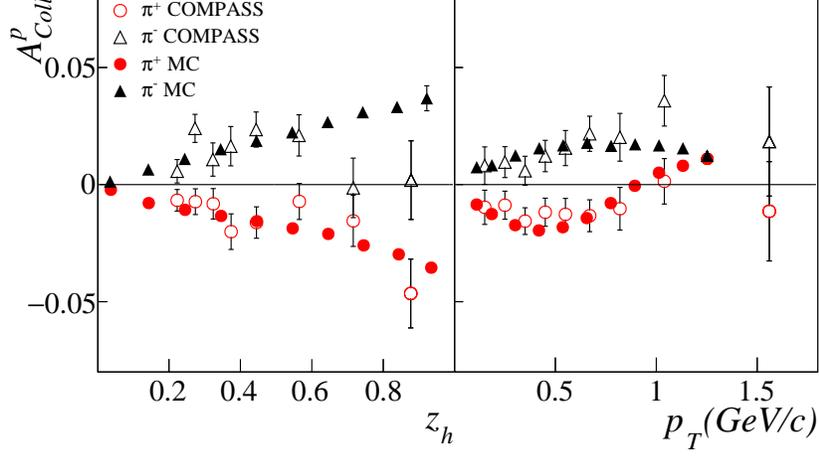
FIG. 11: Comparison between the Collins asymmetry  $A_{Coll}^p$  measured by COMPASS [26] (open points) and the Monte Carlo analysing power  $a^{u \rightarrow \pi^{\pm} + X}$  scaled by  $\lambda$  (full points): as function of  $z_h$  (left panel) and of  $p_T$  (right panel). The cuts  $p_T > 0.1 \text{ GeV}/c$  and  $z_h > 0.2$  have been applied in both cases.
