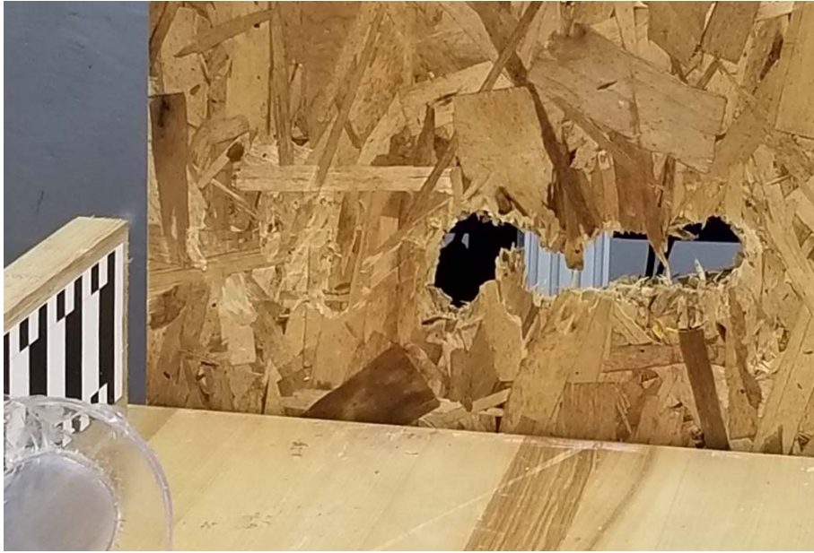
Figure 10 – 15.88mm (5/8 inch) OSB Target
