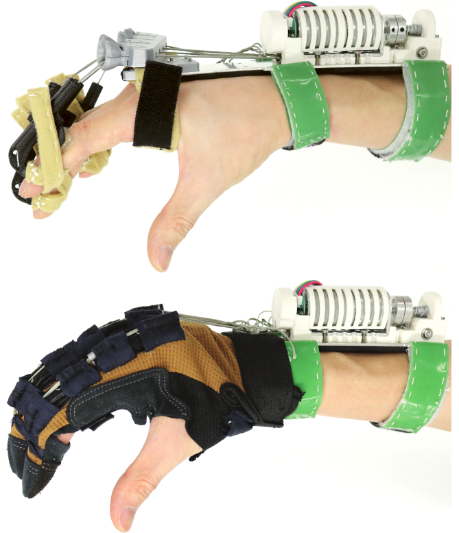
Fig. 1. Prototypes of the hand orthosis transmission mechanisms (top: Design A, bottom: Design B) proposed in this study.
