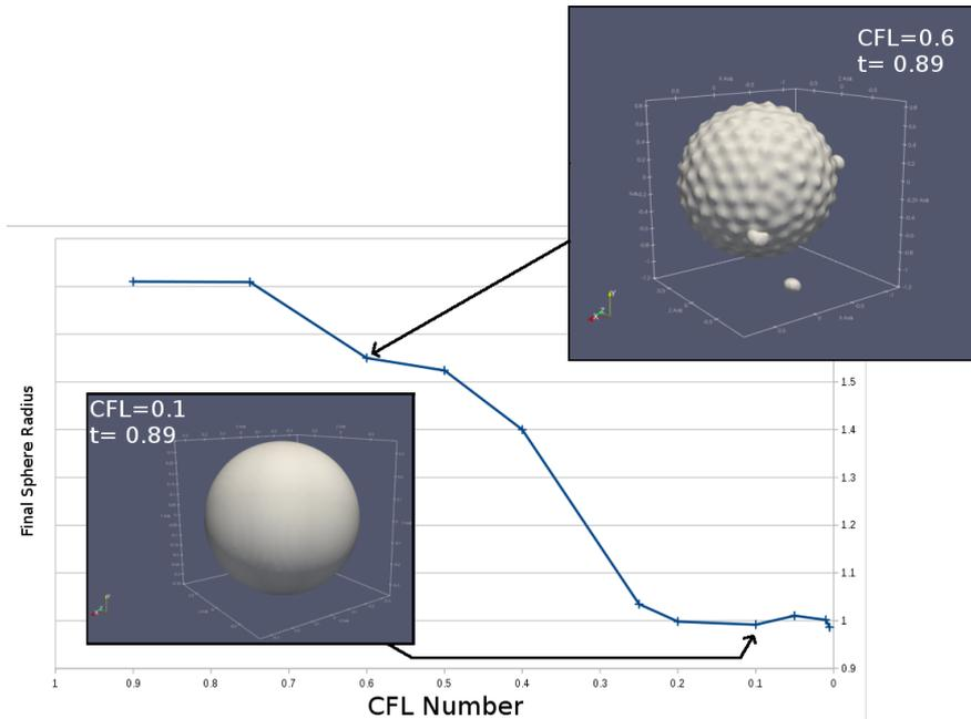
Figure 2: Demonstration of convergence as a function of CFL number. Simulation is unstable for  $CFL > 0.25$ , resulting in visible instabilities in the surface of the simulation.
