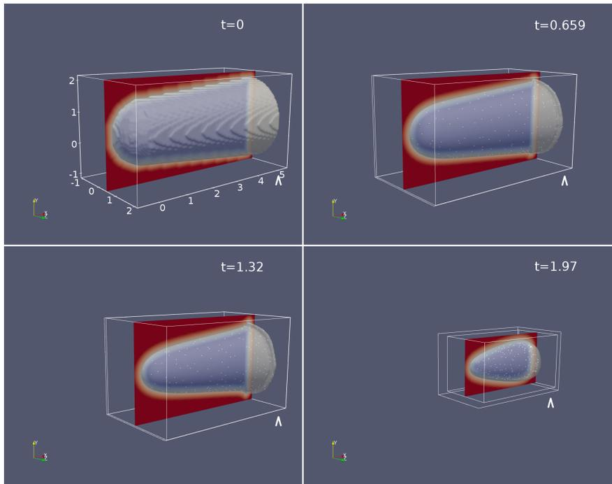
Figure 5: Simulation of truncated tip fixed boundary condition at the truncated end, undergoing curvature flow, total time to complete simulation is 213 s. In this case, the tip correctly shrinks at only one end, however numerical instabilities are visible near the truncated end, and the sides of the tip are removed too quickly as compared to an atom probe experiment, due to the curvature approximation to the Poisson equation.
