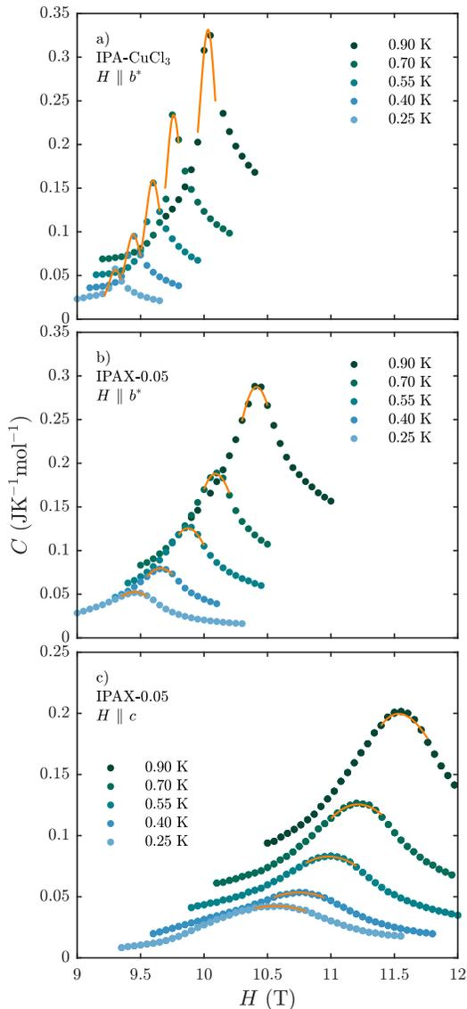
FIG. 2. Specific heat vs. applied field, as measured in IPA-CuCl<sub>3</sub> (a) and IPAX (b,c). The field is almost parallel to the anisotropy axis in (a,b), and almost perpendicular to it in (c). Solid lines are empirical fits to locate the maximum.
