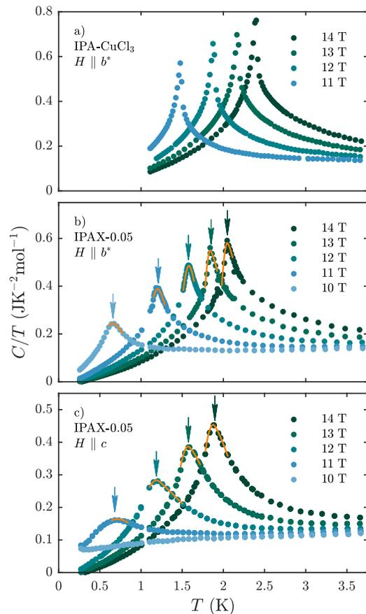
FIG. 1. Magnetic specific heat vs. temperature measured in IPA-CuCl<sub>3</sub> (a) and IPAX (b) for a field applied almost parallel to the anisotropy axis, and IPAX in a field almost perpendicular to it (c). Solid lines are empirical fits to locate the maximum.
