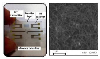
Fig. 1. (a) Inkjet-printed coated SH-SAW device with sensitive layer of DWNTs and (b) SEM image of the printed DWCNTs.
