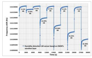
Fig. 6. Real-time detection of different concentrations of humidity.
