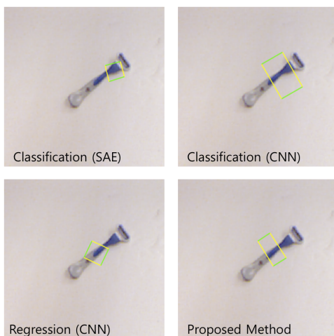
Fig. 10. Four comparison results from classification based grasp detection using sliding window with SAE and CNN, regression based grasp detection and the proposed classification based grasp detection using multi-stage STN.
