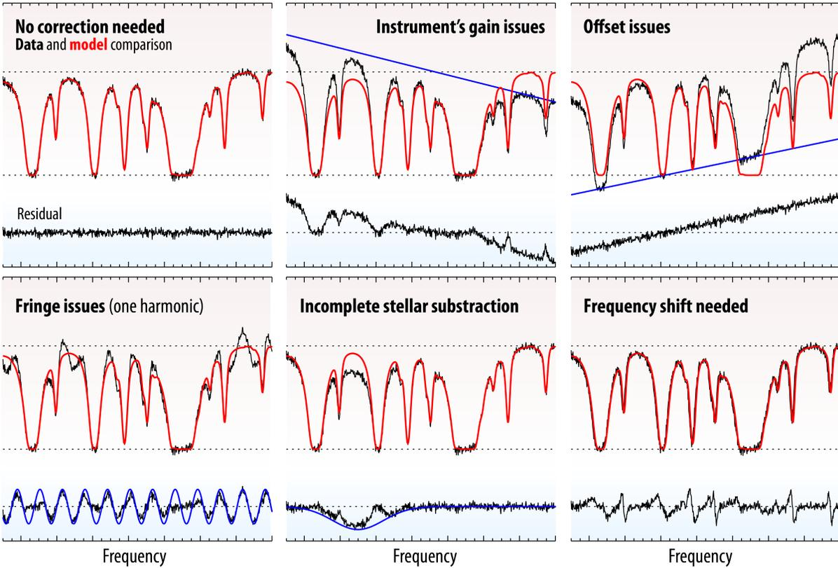
**Figure 8:** Beyond performing the retrieval of planetary parameters, PSG can also correct for several typical issues affecting spectroscopic data. The different panels show how these issues could affect the data, and their impact on the residuals. The methods employed to remove these instrumental effects are described in [92].
