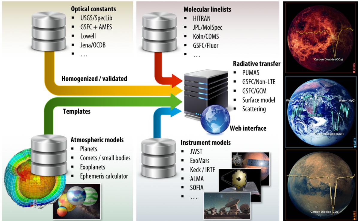
**Figure 1:** The Planetary Spectrum Generator (PSG) integrates a broad range of spectroscopic, atmospheric and instrument databases which are ingested by a versatile radiative transfer suite. By providing a user-friendly web interface to these models and databases, the tool can be utilized to synthesize broad range of planetary spectra. Right panel spectra based on [20] and ESA/Medialab.
