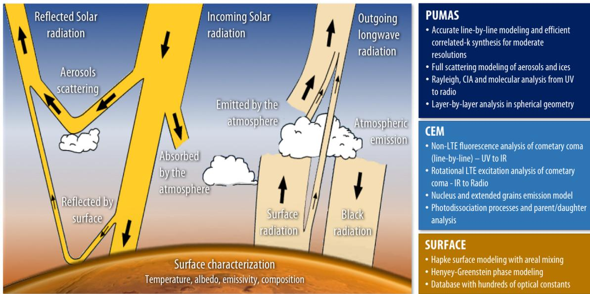
**Figure 5:** The diagram shows the different components considered by the radiative transfer modules. By performing a layer-by-layer analysis, PUMAS integrates and calculates the different flux contributions across the wavelength grid and atmosphere. For comets, the molecular calculation is performed separately by CEM from the surface fluxes, and later added to compute integrated fluxes.
