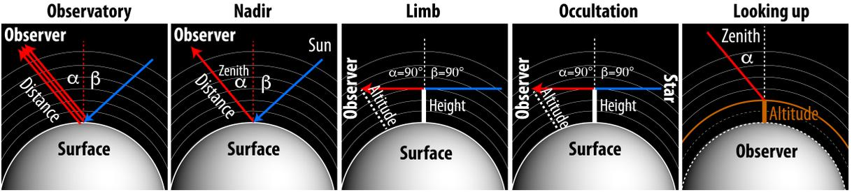
**Figure 2:** Types of geometries considered by PSG. Two main geometry parameters define the viewing configuration for each geometry: incidence angle ( $\beta$ ) and emission ( $\alpha$ ) angles for the observatory and nadir geometries; orbiter altitude and tangent height (i.e., impact parameter) for the limb and occultation geometries; observer’s altitude (with respect to the planetary surface) and zenith angle for the “looking-up” geometry.
