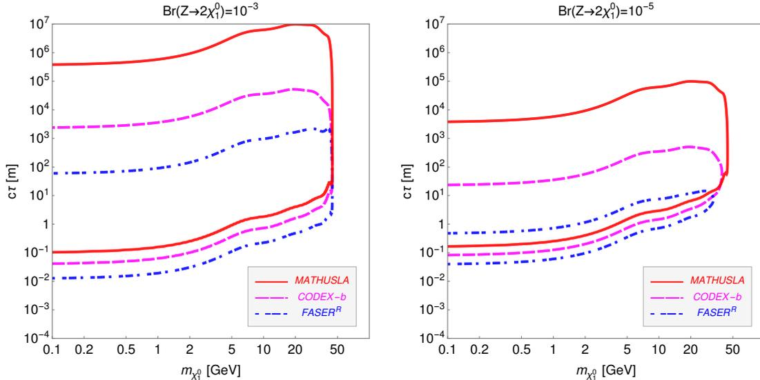
**Figure 5:** Parameter space accessible for CODEX-b, FASER<sup>R</sup> and MATHUSLA for the lightest neutralino in R-parity violating SUSY. This calculation assumes neutralinos are pair-produced from Z-boson decays. The plot on the left assumes  $\text{Br}(Z \rightarrow \chi_1^0 \chi_1^0) = 10^{-3}$  (i.e. a value saturating the experimental upper limit), the one on the right uses  $10^{-5}$ .
