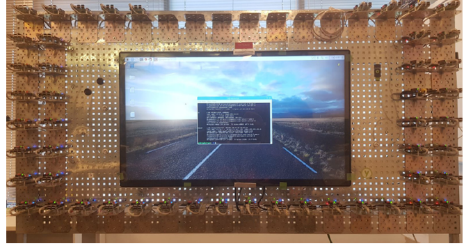
Fig. 3. IoT simulation testbed consisting of 48 Raspberry Pis
