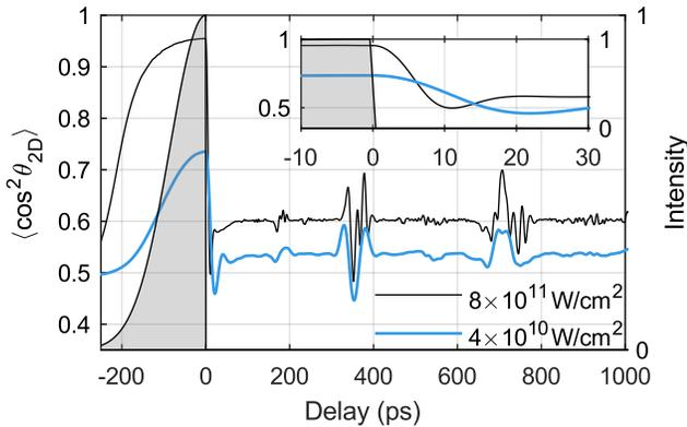
FIG. 4. Calculated values of  $\langle \cos^2 \theta_{2D} \rangle$  with a  $<200$  fs rapidly truncated alignment pulse with peak intensity of  $8 \times 10^{11} \text{ W/cm}^2$  (thin black line),  $4 \times 10^{10} \text{ W/cm}^2$  (thick blue line).
