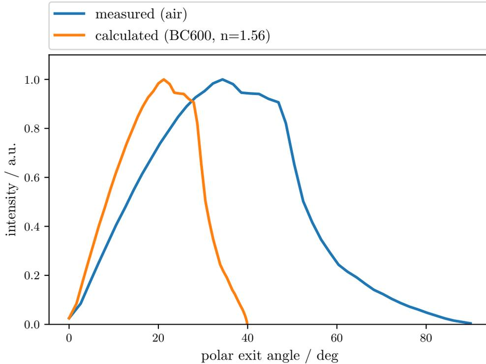
**Figure 5:** The angular distribution of the light output of the used optical fibers. The blue curve shows the measurement in air and the orange curve the corresponding calculation using Snell’s law for the transition from air to Saint-Gobain BC-600 glue [17].
