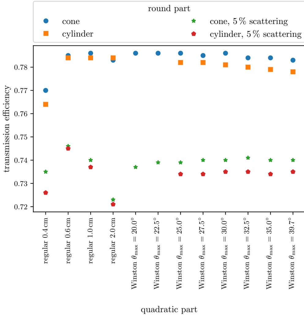
**Figure 6:** The total light guide transmission efficiency for 37 fibers and light guides with an entry-window radius of 4.7 mm to allow a slight misalignment. The simulation is performed for light guides with an ideal surface and for light guides with 5 % Lambertian scattering.
