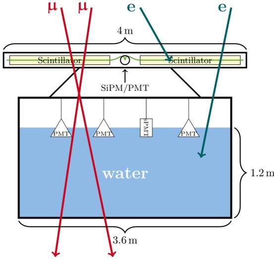
**Figure 21:** A sketch of a Pierre Auger Detector Station after deployment of the SSD. The SSD is mounted on top of the water-Cherenkov detector and detects both the electromagnetic and the muonic shower component. According to the baseline design, it is read-out with a PMT. For test purposes, three detectors are equipped with a SiPM module.
