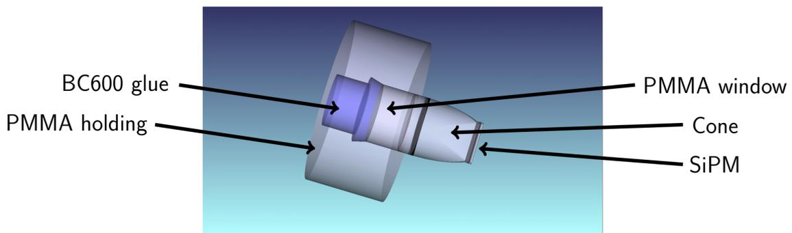
**Figure 4:** The basic design for the simulation. All optical components including the Saint-Gobain BC-600 optical cement, the PMMA holding structure and the reflective aluminium ring are implemented. Only one fiber bundle is simulated because the distance between the two fiber bundles is large enough to be optically independent.
