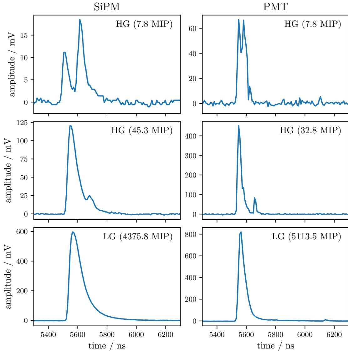
**Figure 27:** The signal traces measured by the neighbouring SiPM and PMT station for three different events. Note that the detectors are not placed on top of each other. Thus, they do not measure exactly the same signal but only the same shower at slightly different locations.
