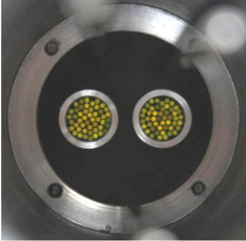
**Figure 2:** A front view of the holding structure for the two fiber bundles as it is already installed inside the detector. Each fiber bundle is surrounded by an aluminium ring. The three blurred pins (two at the top, one at the bottom) allow to precisely position the SiPM module in front of the fiber bundles.
