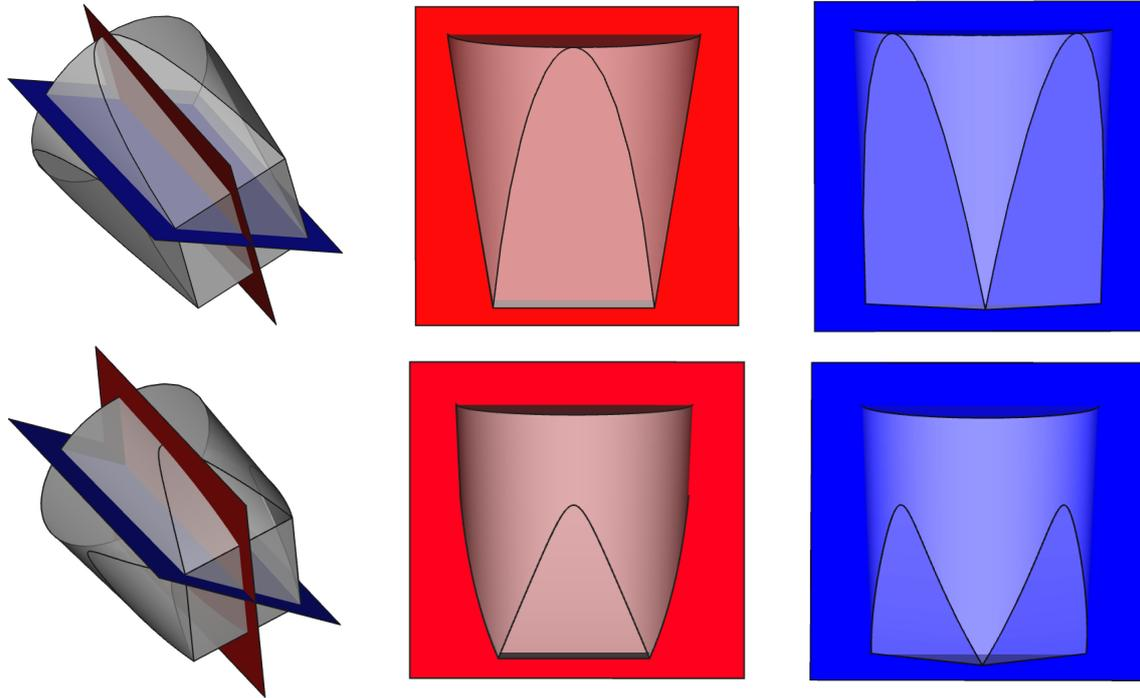
**Figure 3:** Examples of the resulting light guide geometries. Both shown light guides will be studied in detail later. *Top row:* A light guide consisting of a regular pyramid and a cone with a length of 1 cm shown from three different perspectives. All surface contours follow straight lines. *Bottom row:* A light guide consisting of a Winston pyramid and a cone with a cut-off angle of  $39^\circ$ . Here, the Winston pyramid causes parabolically shaped surface contours.
