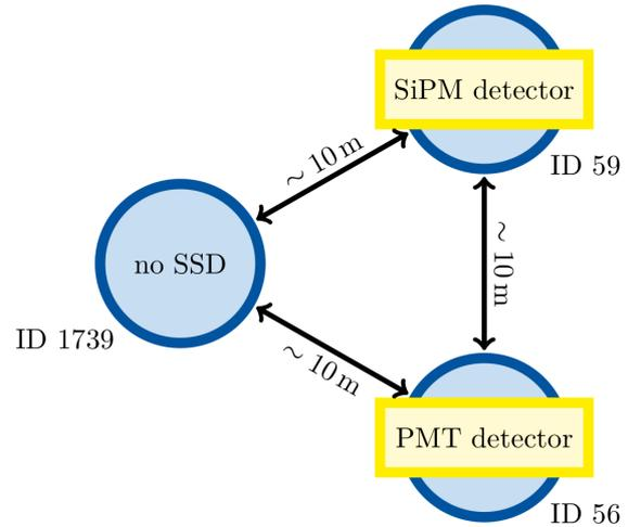
**Figure 22:** A schematic view of the station layout at the detector station equipped with a SiPM module. One neighbouring station is equipped with an SSD with a PMT and a third station is not equipped with an SSD. A unique ID identifies the stations.
