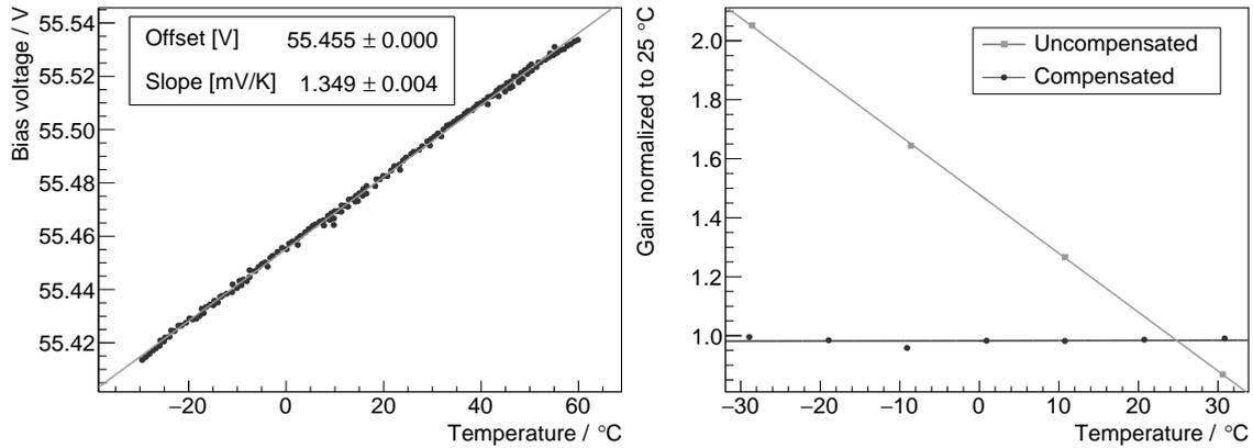
**Figure 18:** *Left:* Intrinsic temperature dependence of the Hamamatsu C11204-02 power supply chip as measured in a climate chamber. *Right:* SiPM gain versus temperature compensated with a linear temperature progression and uncompensated with a constant bias voltage.
