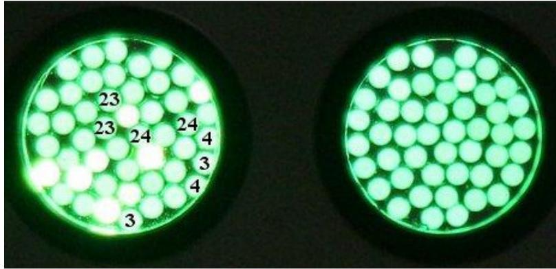
**Figure 15:** The two fiber bundles for the detector shown in figure 14. The left side corresponds to the top half ( $y=2.2$  to  $3.7$  m) of the detector. The fibers labelled 3 and 4 correspond to the bars at the very right of the detector. The fibers labelled 23 and 24 correspond to the bars at the left of the detector.
