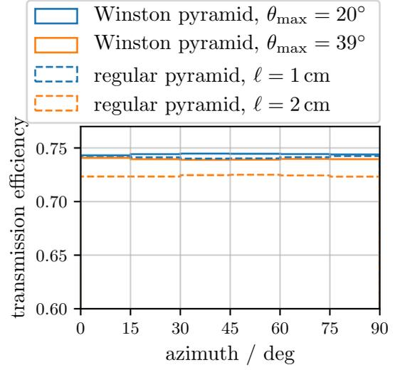
**Figure 9:** Mean efficiency depending on the azimuth angle  $\varphi = \arctan(y/x)$ . Only radial distances up to the maximum of 3.5 mm are taken into account. The distribution is flat for all tested geometries.
