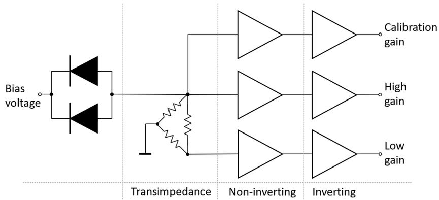
**Figure 19:** This figure shows the schematic overview of the pre-amplifier architecture used in the latest revision of the printed circuit board. Two SiPMs are connected in parallel and read-out by a simple resistor bridge (transimpedance stage) with a total impedance of  $50\ \Omega$ . A non-inverting current feedback stage is followed by an inverting stage forming three individual amplifier channels.
