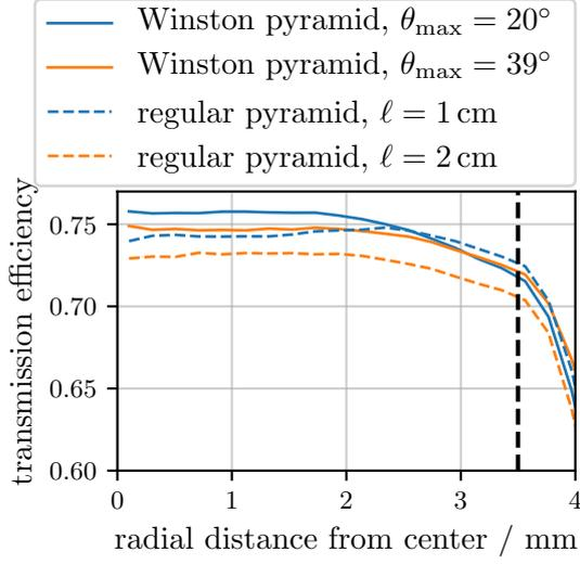
**Figure 8:** Mean efficiency depending on the radial distance of the fiber from the center for different light guide geometries. The dashed vertical line denotes the maximum radial distance a fiber can have inside the cookie.
