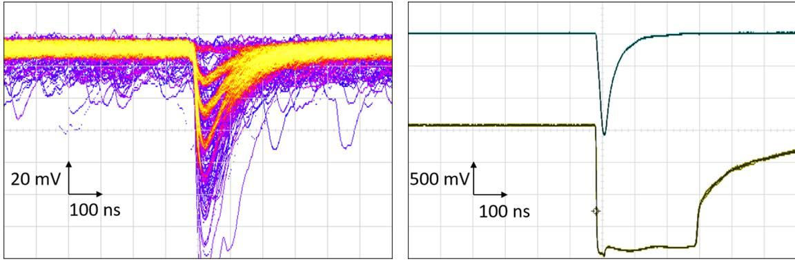
**Figure 20:** *Left:* Two  $6 \times 6 \text{ mm}^2$ -sized,  $25 \mu\text{m}$  cell pitch SiPMs amplified by the calibration channel flashed by and triggered on an LED with 1 s persistence. *Right:* Large-signal response ( $>90\,000 \text{ p.e.}$ ) of the high-gain and the low-gain channel using a pulsed LED. No undershoot or oscillation can be observed even though the high-gain and inevitably also the calibration channel are clearly saturated.
