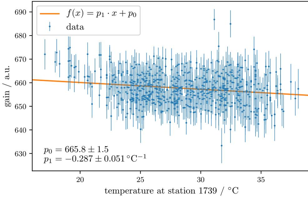
**Figure 24:** The gain of the SiPM with respect to the temperature. At the time of data taking, the read-out of monitoring values such as temperature was not yet implemented for the new detectors. Thus, the temperature was taken from the old station 1739 which is  $\sim 10$  m apart.
