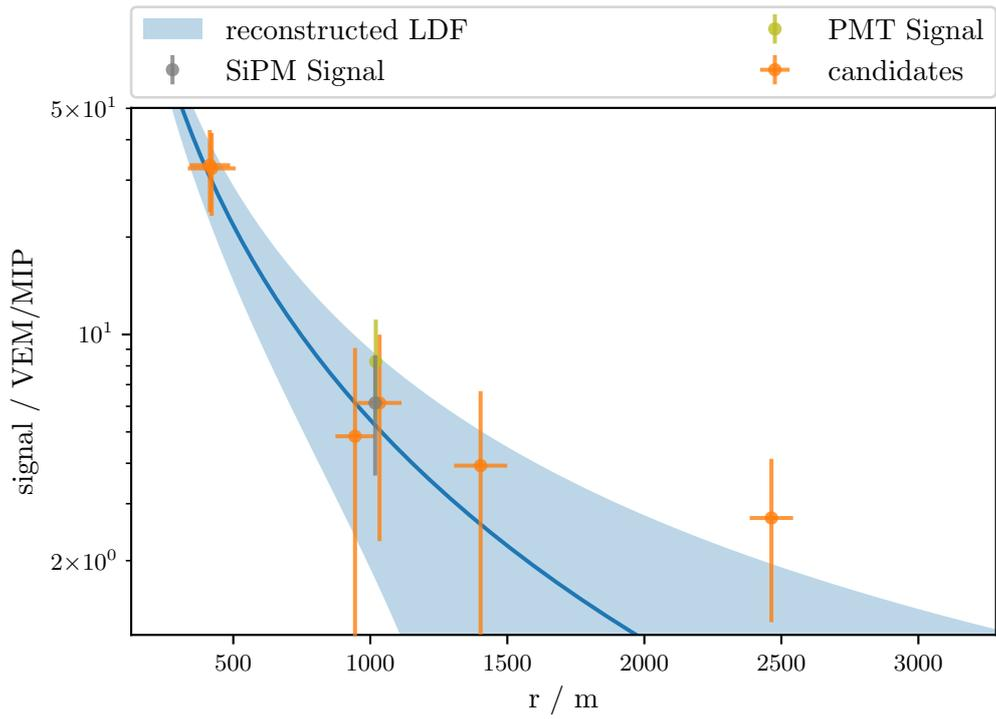
**Figure 28:** The LDF reconstructed from the signals measured in the surface detector stations. The blue band gives the  $1\text{-}\sigma$  uncertainty region of the reconstruction. The corresponding signal traces for the PMT and SiPM, respectively, are shown in the top row of figure 27. The signals in the two SSDs are in agreement with each other and also with the reconstructed LDF.
