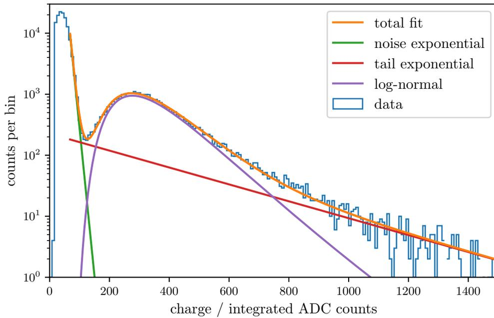
**Figure 25:** An example of a calibration histogram measured with the high-gain channel of the SiPM module. Here, the MIP peak is visible and well separated from the noise. The shown fit consists of three components. First, an exponential function describing the exponential SiPM noise background; second, an exponential to describe the tail of the distribution; third, a log-normal distribution to fit the peak.
