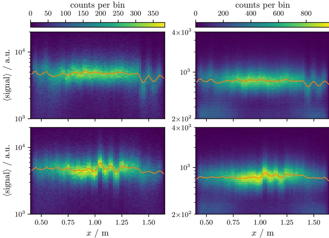
**Figure 16:** The signal distribution for different positions along the width of the detector as shown in figure 14. The *left* plots correspond to the measurement with the SiPM module, the *right* ones to that with the PMT. The *top* and *bottom* row show the signal for the two detector halves, respectively. Different scintillator bars can be identified because of the varying light yield. The median of the distribution is denoted by an orange line.
