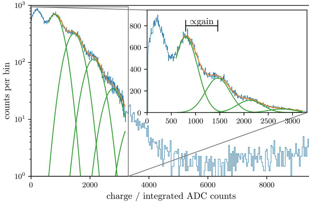
**Figure 23:** An example of a calibration histogram measured with the calibration-gain channel of the SiPM module. Due to the limited range of the histogram, the MIP peak at  $>30$  p.e. is not visible here. Peaks corresponding to a single p.e. are well visible and allow determination of the SiPM gain.
