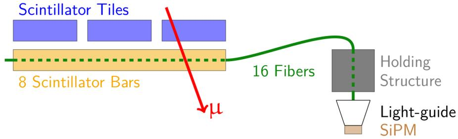
**Figure 12:** Schematic of the setup for determining the different performances of the light guides. The light produced in scintillator bars by through-going atmospheric muons is collected in WLS fibers and guided onto the light guide under test. It is read out with a SiPM and triggered by external scintillators.
