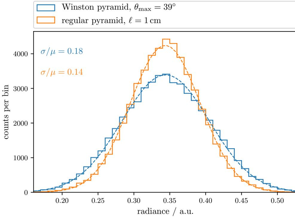
**Figure 11:** The spatial homogeneity of the illumination of the SiPM for two different light guide geometries. The simulation statistics is the same for both light guides. The simulated distributions show good agreement with Gaussian fits.  $\sigma$  and  $\mu$  refer to the Gaussian width and mean of the distribution, respectively.
