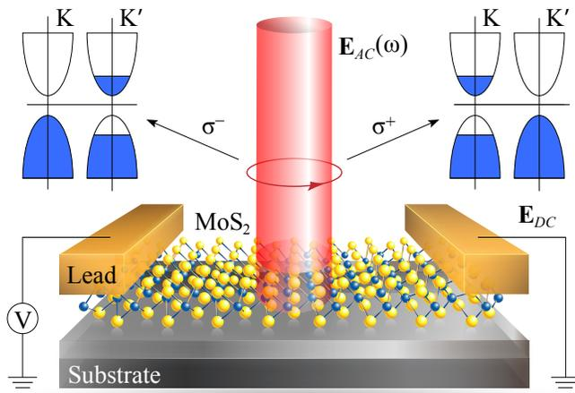
FIG. 1: Schematic of EMF-induced Hall transport in a 2D Dirac semiconductor (monolayer MoS<sub>2</sub>).  $\mathbf{E}_{DC}$  is a probe field (bias), and  $\mathbf{E}_{AC}$  is an external electromagnetic wave of light that can be right- or left-circular polarized. Depending on the polarization, either  $K$  or  $K'$  valleys couple to light.
