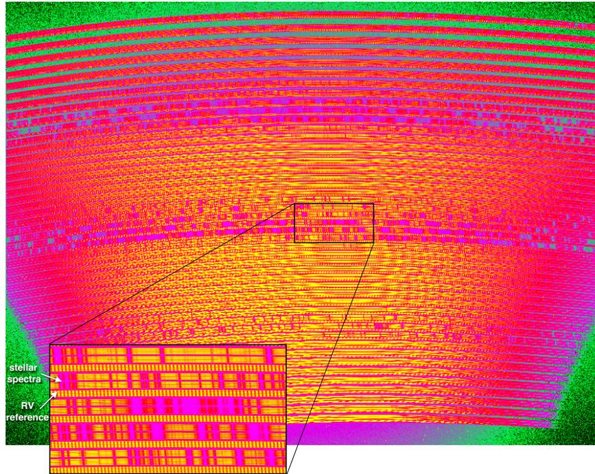
**Fig. 8** Simulated raw SPIRou stellar frame, with a close up on the central part of orders #53 to #57. The two stellar spectra of each order correspond to the orthogonal states of the selected polarisation, whereas the third spectrum tracks the Fabry-Perot RV reference. All three spectra feature four identical slices.
