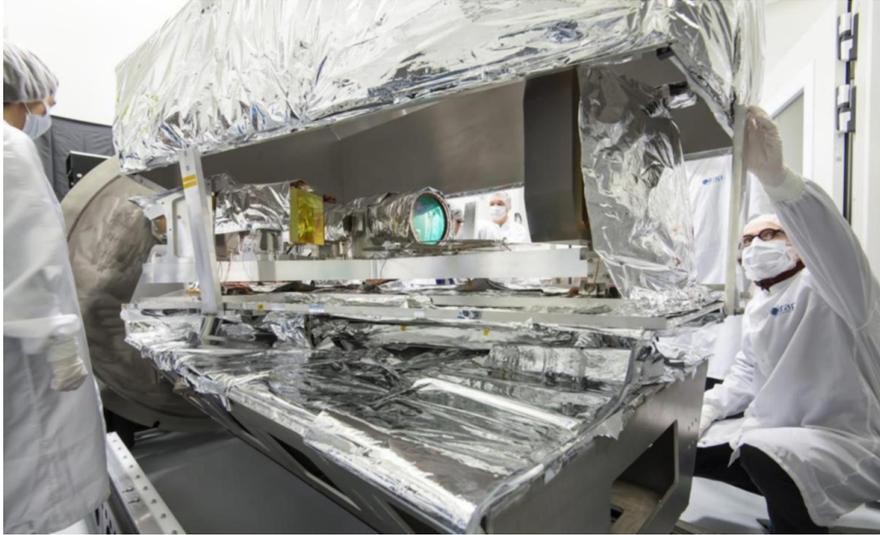
**Fig. 10** Closing the SPIRou cryostat prior to the second cool-down cycle, with the spectrograph bench hosting its full optical load (© S Chastanet, IRAP/OMP).
