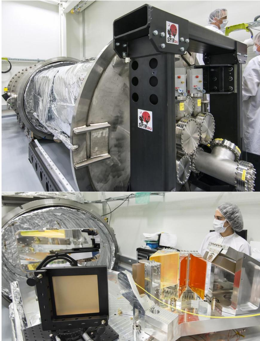
**Fig. 9 Top panel:** Preparing for a SPIRou cryostat cool-down phase in the SPIRou clean room. **Bottom panel:** Aligning the spectrograph optics on the bench while waiting for the spectrograph camera to reach IRAP / OMP; the grating, the prism train and the folding mirror are in the front, right-hand side, whereas the large parabolic collimator is in the rear, left-hand side (© S Chastanet, IRAP/OMP).
