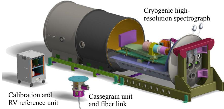
**Fig. 4** CAD view of the main SPIRou units.
