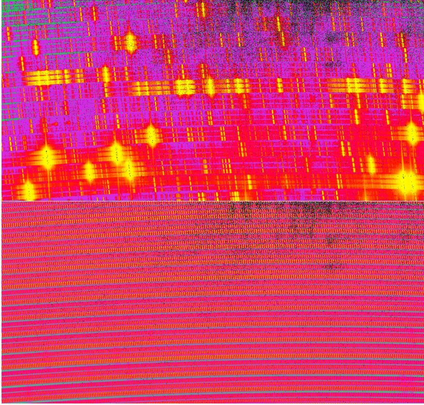
**Fig. 11** Blue orders of UNe hollow-cathode (top panel) and Fabry-Perot etalon (bottom panel) spectra recorded by SPIRou during the third thermal cycle in 2017 June, when the spectrograph detector was located only 50  $\mu\text{m}$  away from the focal plane.
