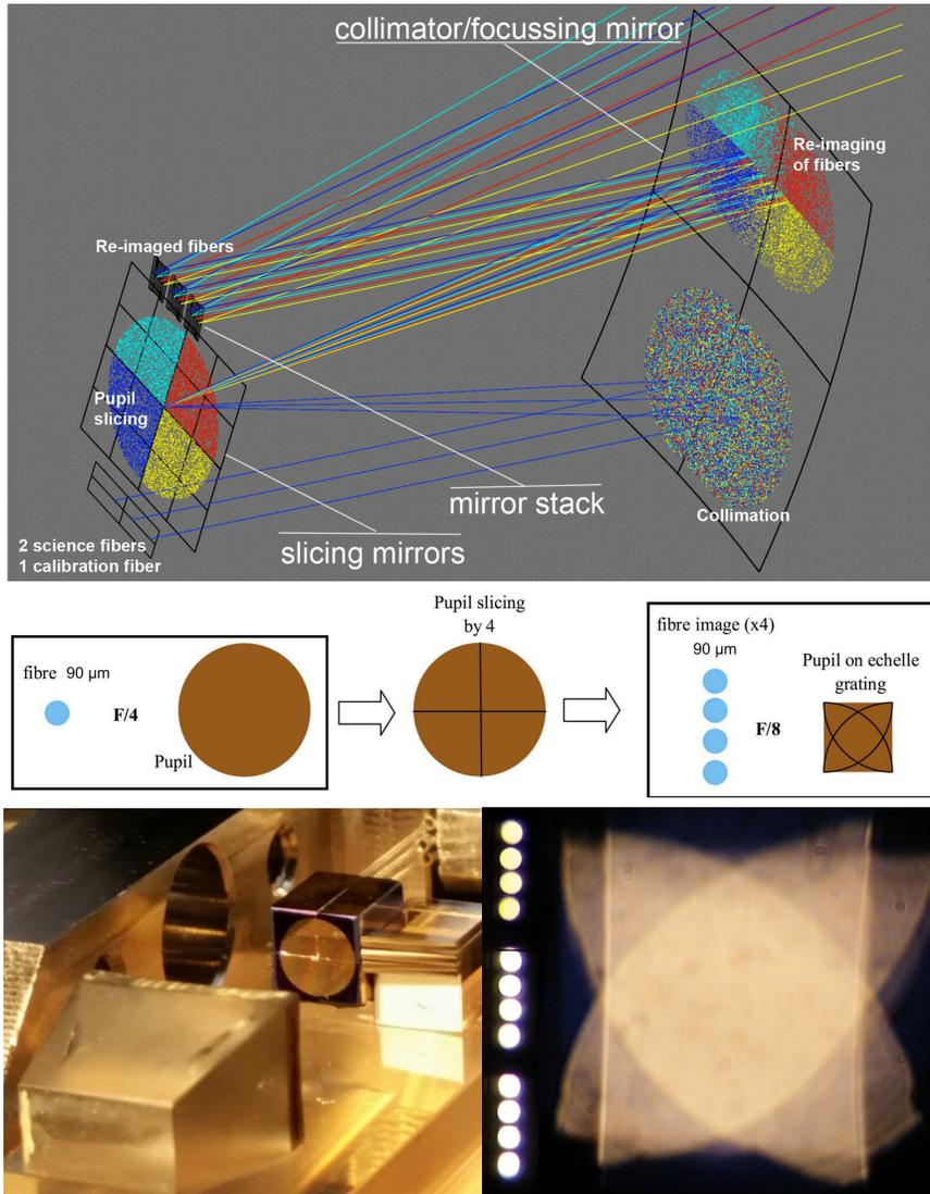
**Fig. 6** Top panel: Optical view of the SPIRou pupil slicer. Middle panel: Schematic view of the pupil slicing principle for a single fibre. Bottom panel: Test pupil slicer assembled by WinLight (left), and corresponding slit / pupil profiles for a slightly oversized beam aperture (right).
