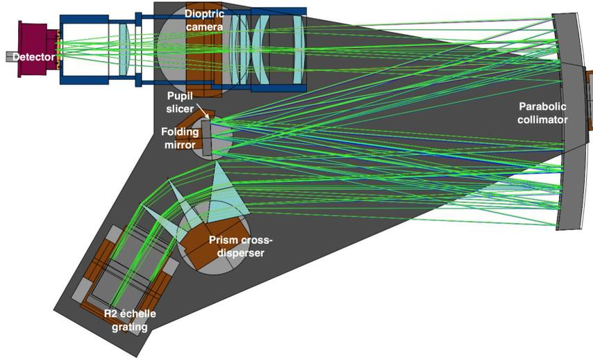
Fig. 7 Optical view of the SPIRou spectrograph.
