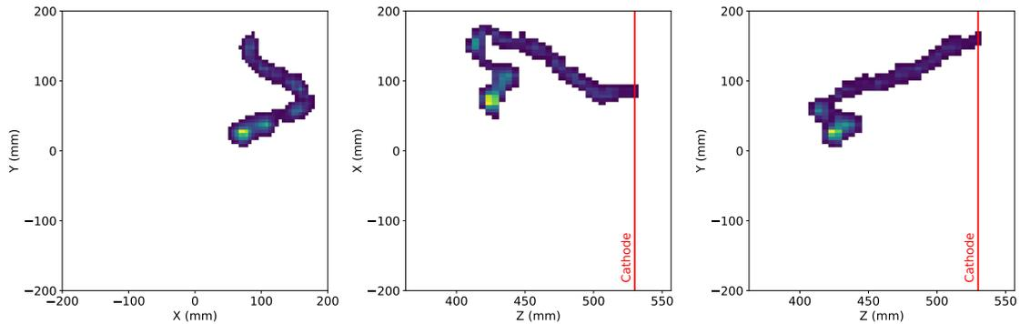
**Figure 8.** High energy ( $E > 1.5$  MeV) electron originating from the cathode. The three projections,  $XY$  (left),  $ZX$  (center) and  $ZY$  (right), show the expected topological signature of an electron.
