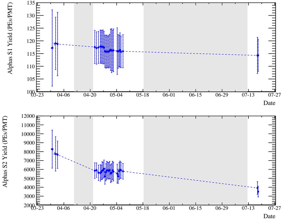
**Figure 5.** S1 (top) and S2 (bottom) yields, corrected for the  $Z$  spatial dependence and for all fiducial alpha events, during run periods A1–A3. The data points and error bars indicate the mean and the RMS of the  $Z$ -corrected distributions, respectively.
