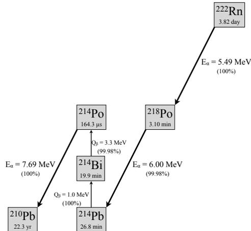
**Figure 1.** Part of the  $^{222}\text{Rn}$  decay scheme that is most relevant for rare event searches.
