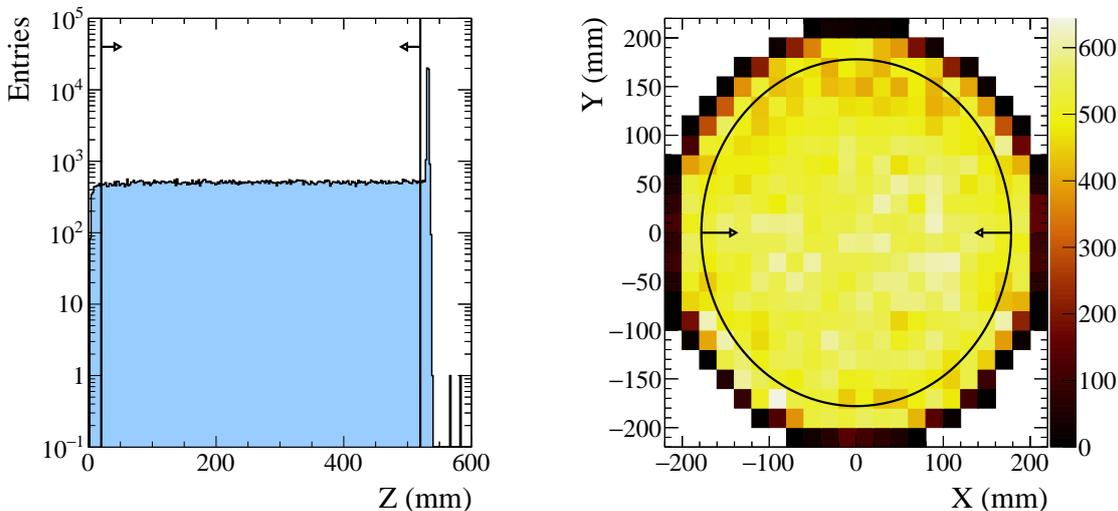
**Figure 2.** Spatial distribution of alpha candidate events. Left panel:  $Z$  distribution. Right panel: distribution in the  $(X, Y)$  plane. In the two panels, the solid black lines and arrows indicate the fiducial region.
