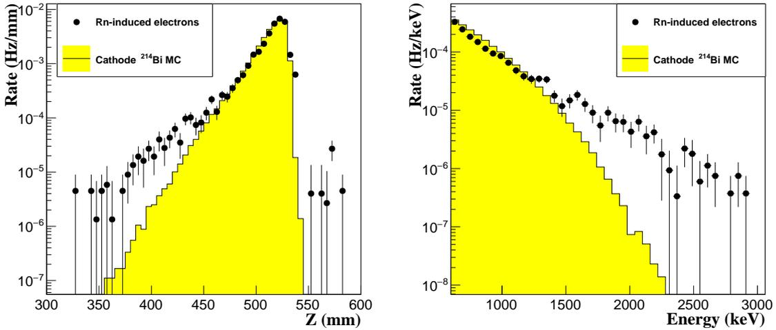
**Figure 9.** Radon-induced electrons originating from the cathode (black dots) superimposed on the MC expectation (yellow histogram), as a function of the reconstructed  $Z$  coordinate (left panel) and reconstructed energy (right).
