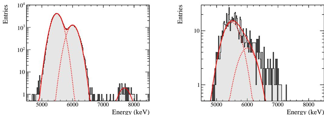
**Figure 6.** Energy distribution for fiducial alpha candidate events during run periods A3 (left panel) and A1 (right panel). A triple gaussian fit is superimposed to the A3 histogram to describe the  $^{222}\text{Rn}$  (5489 keV),  $^{218}\text{Po}$  (6002 keV) and  $^{214}\text{Po}$  (7687 keV) populations. Only the  $^{222}\text{Rn}$  and  $^{218}\text{Po}$  yields are fitted in the A1 histogram.
