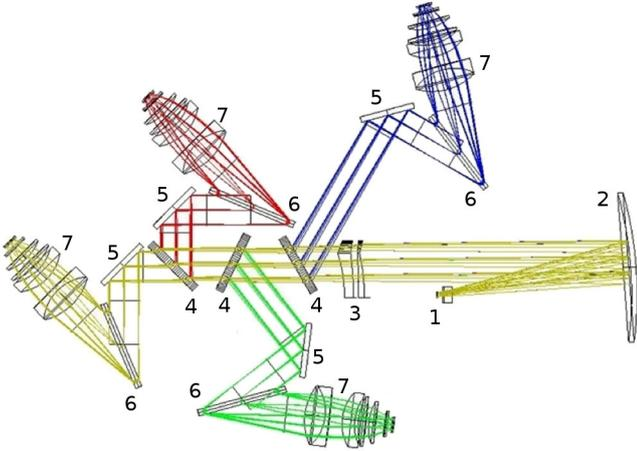
**Figure 1.** Schematics of the Hermes spectrograph. 1: Slit assembly, 2: Collimator, 3: Corrector, 4: Beam splitters, 5: Fold mirrors, 6: Gratings, 7: Camera and CCD assemblies. Blue, green and red rays mark the respective arms and yellow rays mark the IR arm.
