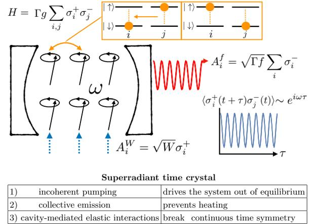
FIG. 1. An ensemble of  $N$  spin 1/2 particles pumped at rate  $W$ , experiencing collective emission at rate  $\propto f\Gamma$  and collective spin-exchange interactions (orange),  $\propto g\Gamma$ , form the basis of the superradiant TC. The elastic interactions imprint collective spin oscillations at frequency  $\omega$  spontaneously breaking the time translation symmetry (manifested as persistent oscillations in the unequal time spin-spin correlation function in the thermodynamic limit).
