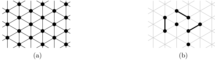
Figure 1: (a) A section of the triangular lattice G_\Delta . (b) Expanded and contracted particles (black dots) on G_\Delta (gray lattice). Particles with a black line between their nodes are expanded.
