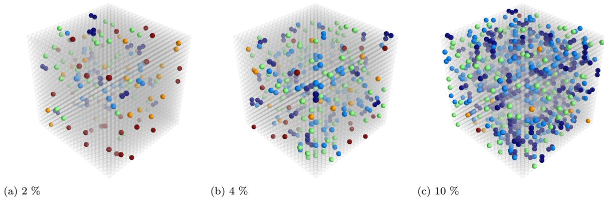
FIG. S2: Examples of the distribution of defects (colored spheres) on an SP lattice with the edge length of  $N = 21$  sites for three selected concentrations  $n$ . The color identifies the defects having the same distance to the nearest neighbor defined in the units of the exchange path  $p_0$ : dark blue  $= p_0$ ; light blue  $= 2p_0$ ; green  $= 3p_0$ ; orange  $= 4p_0$ , and red  $\geq 5p_0$ . (see the text)
