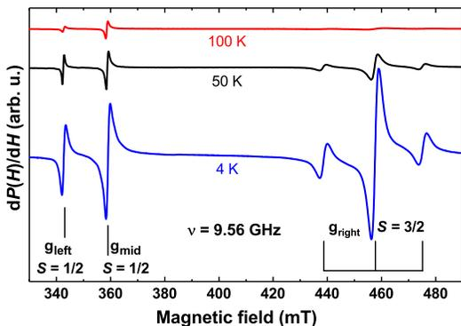
FIG. 1. ESR spectra (field derivatives of absorption) at the X-band frequency  $\nu = 9.56$  GHz at three selected temperatures. The lines at  $\sim 340$  mT and  $\sim 360$  mT, and a triplet structure centered around  $\sim 460$  mT are labeled as  $g_{\text{left}}$ ,  $g_{\text{mid}}$ , and  $g_{\text{right}}$ , respectively, with the spin values assigned to each line.
