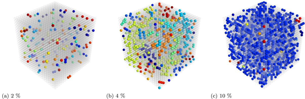
FIG. S3: Examples of the clustering of defects (colored spheres) on an SP lattice with the edge length of  $N = 21$  sites with increasing their concentration  $n$ . The defects are connected in a cluster by the maximum exchange path length of  $2p_0$ . Defects belonging to the same cluster have the same color. (a)  $n = 2\%$ , practically all defects are independent; (b)  $n = 4\%$ , defects are coupled in mid-size clusters; (c)  $n = 10\%$ , practically all defects belong to the same cluster.
