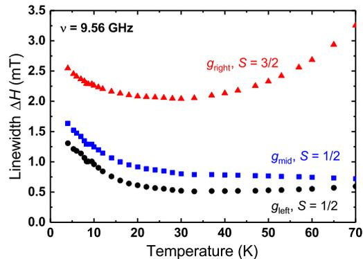
FIG. 4.  $T$  dependence of the width  $\Delta H$  of the ESR signals  $g_{\text{left}}$ ,  $g_{\text{mid}}$  and  $g_{\text{right}}$  (main peak) at  $\nu = 9.56$  GHz.
