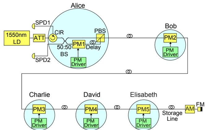
FIG. 4. Single-qubit QSS (reprinted from Ref. 5). Alice randomly modulates the state, adding a phase of 0 or  $\pi/2$ . The rest of parties randomly choose a phase from  $\{0, \pi/2, \pi, 3\pi/2\}$ . Here, LD denotes a laser diode, ATT denotes an attenuator, SPD denotes a single-photon detector, CIR denotes a circulator, BS denotes a beam splitter, PBS denotes a polarization beam splitter, PM denotes a phase modulator, AM denotes an amplitude modulator, FM denotes a Faraday mirror.
