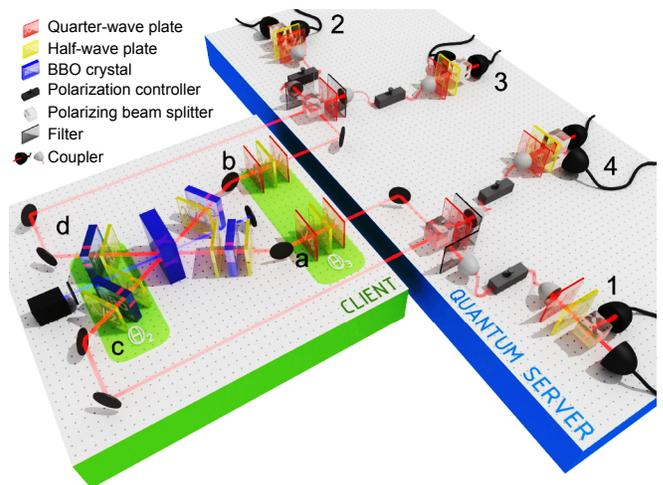
FIG. 7. Proof-of-principle implementation of BQC (reprinted from Ref. 19). Entangled photon pairs are generated from non-collinear type-II spontaneous parametric down-conversion process in BBO crystal. The horizontal and vertical polarization represents  $|0\rangle$  and  $|1\rangle$ .
