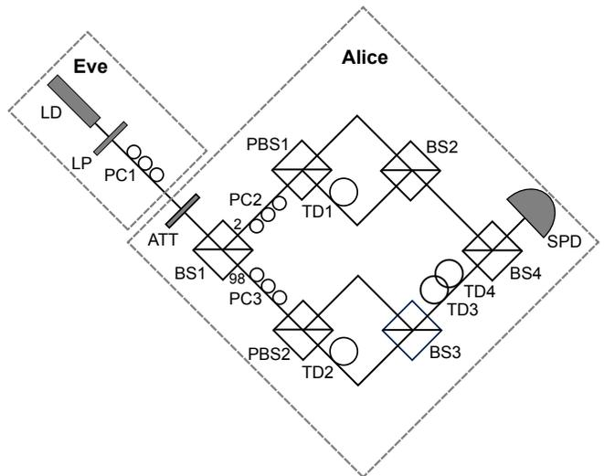
FIG. 5. Experimental scheme for SI QRNG (reprinted from Ref. 17). The untrusted party Eve prepares quantum states and sends them to Alice, who is trusted. Alice then generates random numbers. Here, LD is a laser diode, LP is a linear polarizer, PC is a polarization controller, ATT is an optical attenuator, BS is a beam splitter, PBS is a polarization beam splitter, TD is a time delay, SPD is a single-photon detector.
