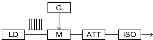
FIG. 8. The scheme of countermeasures against source imperfections. To eliminate the mismatch among different laser diodes, a single laser diode LD followed by a modulator M can be used. The following attenuator ATT and isolator ISO provide sufficient isolation to prevent the Trojan-horse attack in a unidirectional system. Here, G denotes a modulation signal generator.
