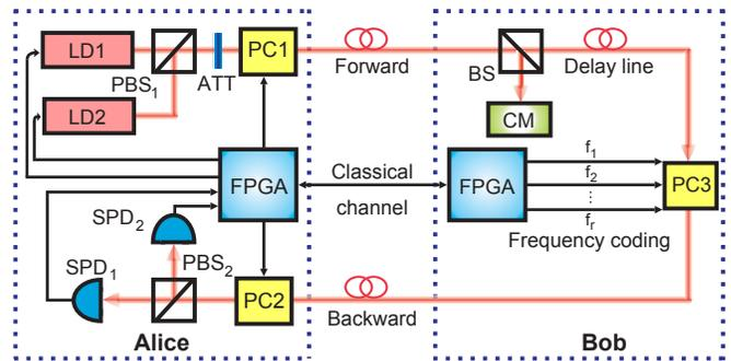
FIG. 6. QSDC implementation (reprinted from Ref. 18). Alice prepares and measures states, and Bob encodes the secret message by manipulating the states. Here, LD is a laser diode, PBS is a polarization beam splitter, ATT is an optical attenuator, PC is a polarization controller, BS is a beam splitter, CM is a control module, FPGA is a field programmable gate array, SPD is a single-photon detector.
