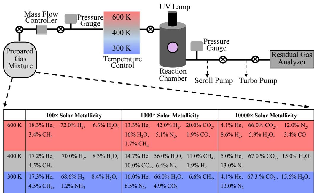
Figure 1. Schematic of the PHAZER setup for current work and the gas mixtures used in the experiments. To be noted, the schematic is shown to provide a concept of our setup, and it is updated from our previous studies to include the new energy source (UV lamp); the gas mixtures used here are the same as our previous plasma experiments (He et al. 2018, Hörst et al. 2018a). The detailed procedure was discussed in He et al. (2018).
