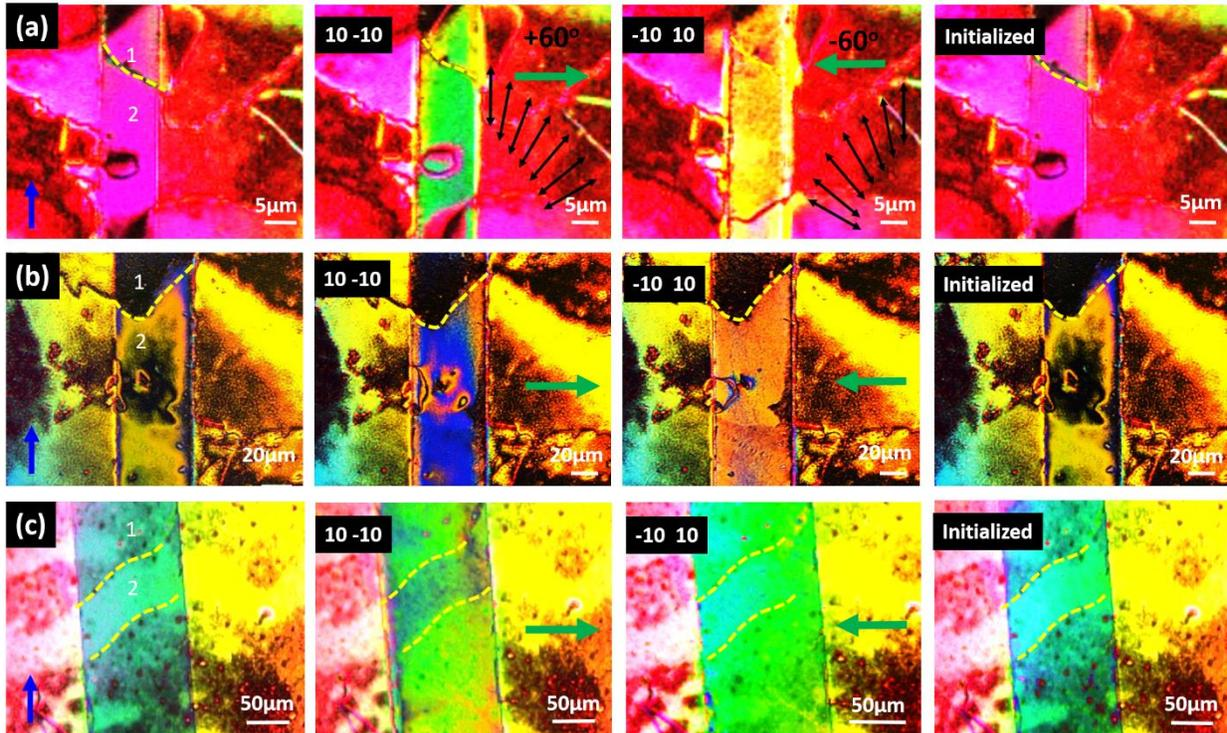
**Figure 3: Controlling three states with dynamic colors by pulse sequence on two electrodes:** Rubbed layer was placed on top with the rubbing direction parallel to the electrodes (blue arrows). Pulses with different field direction (marked with green arrows) were applied to reorient LC
