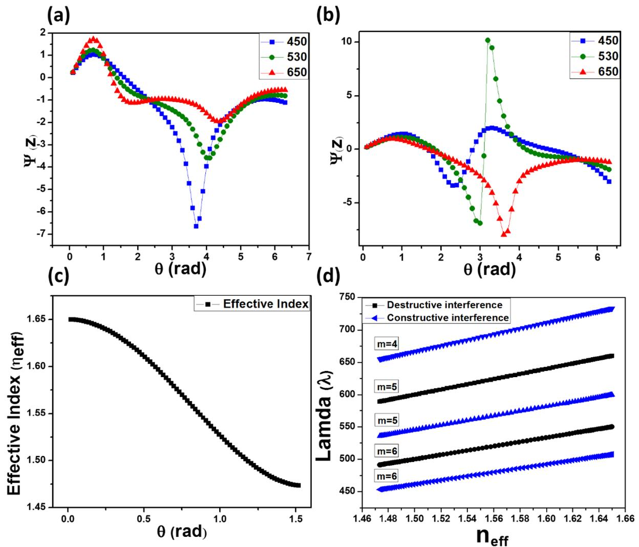
**Figure 4: Theoretical estimation of transmittance as function of twist angle:** (a-b) Relation between transmittance and twisted angles was plotted for various wavelengths ( $\lambda = 450, 530,$  and  $600$  nm), for the cells with widths (a)  $2 \mu\text{m}$  and (b)  $3 \mu\text{m}$ , respectively. The wavelength with
