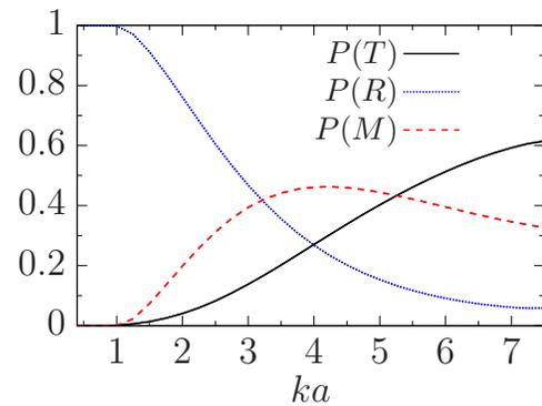
FIG. 2. Transmission and reflection coefficients of dimers as well as the monomer production coefficient (defined in the main text) for an input unidirectional dimeric wave, as a function of  $ka$ . The other parameters are the same as in Fig. (1).
