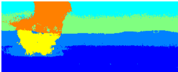
FIGURE 4. Segmentation of a hyperspectral video using graph MCF. The gas plume is clearly represented in the yellow and orange pixels. The two blue communities on the bottom are the ground, and the other two communities are the sky. This image is frame 3 of 7. (It is best to view this plot in color.)
