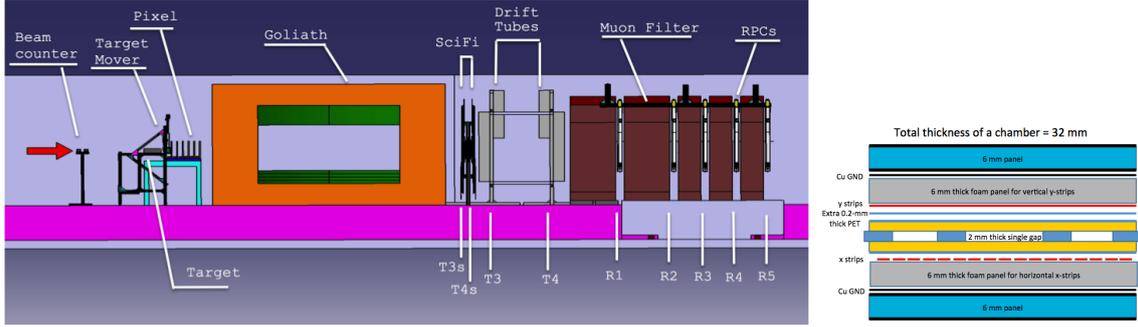
**Figure 4.** Left: Setup of the charm measurement experiment including the downstream muon filter based on the RPC technology. Right: structure of the 32 mm thick RPC chamber.
