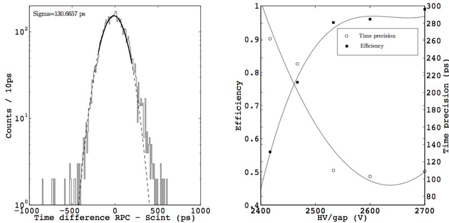
**Figure 5.** Left: Distribution of the time difference between one of the reference scintillators and the prototype chamber after the walk correction. Right: Time accuracy and efficiency as a function of the HV/gap.
