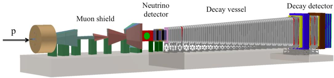
**Figure 1.** The beam dump facility and the SHiP detector.
