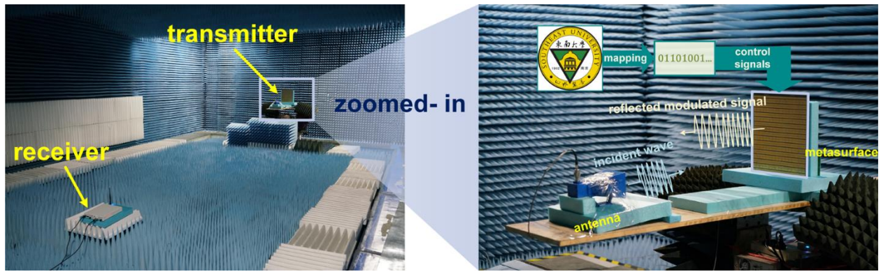
Figure S8. The photograph of the experimental setup for the new BFSK wireless communication system.
