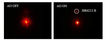
Fig. 8: HR 6212 A/B images before and after PAO correction at 3.5-meter ARC telescope.
