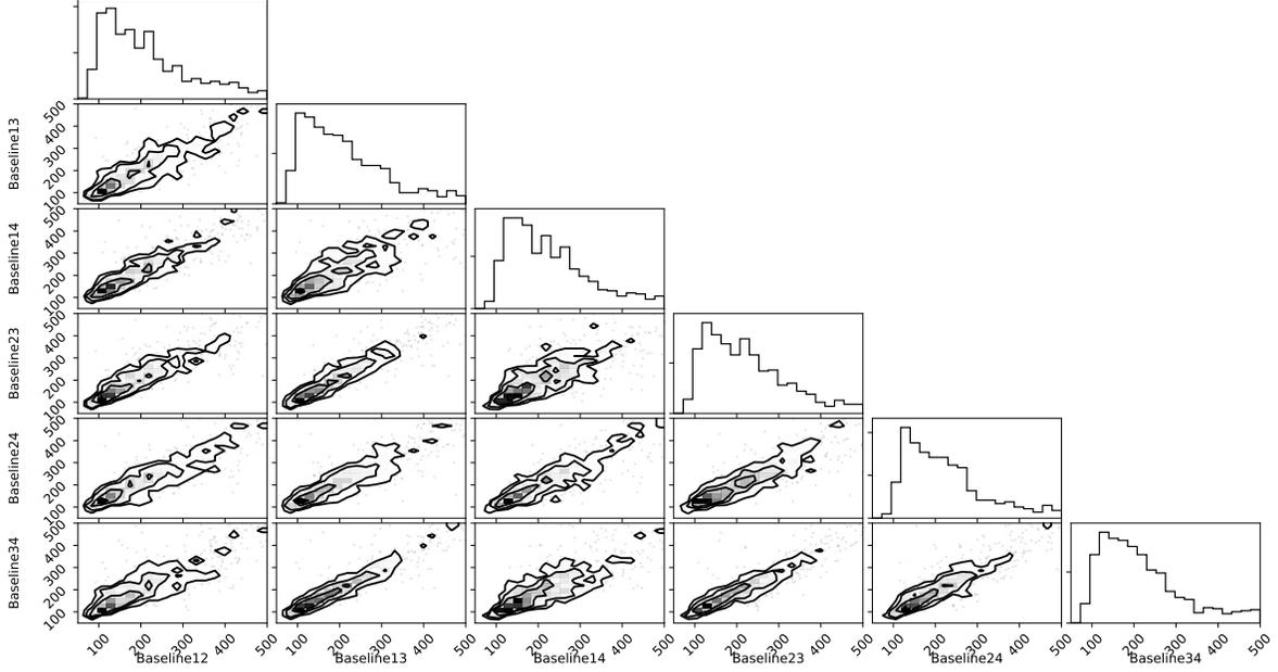
Figure 1. Correlation between the OPD residual error (in nanometers) observed on the different baselines. The residuals are obtained from the calibrators observed between June 2016 and October 2017. The median tracking residual is 180 nm.
