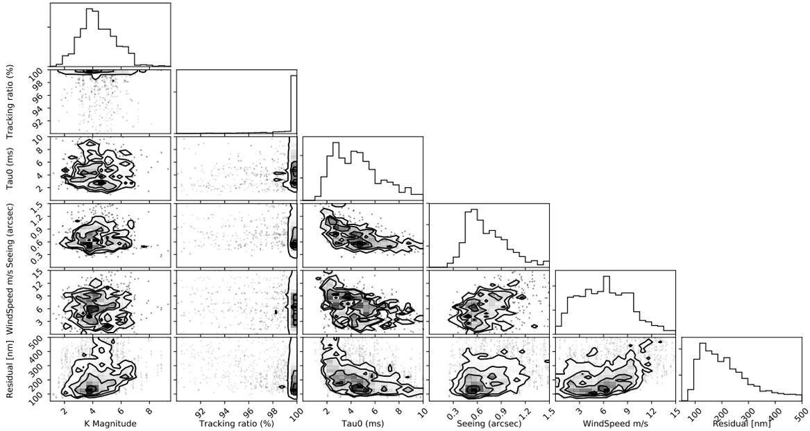
Figure 2. Correlations between OPD residuals, K magnitude, tracking ratio, coherence time, seeing and wind speed (from the Paranal ASM system).
