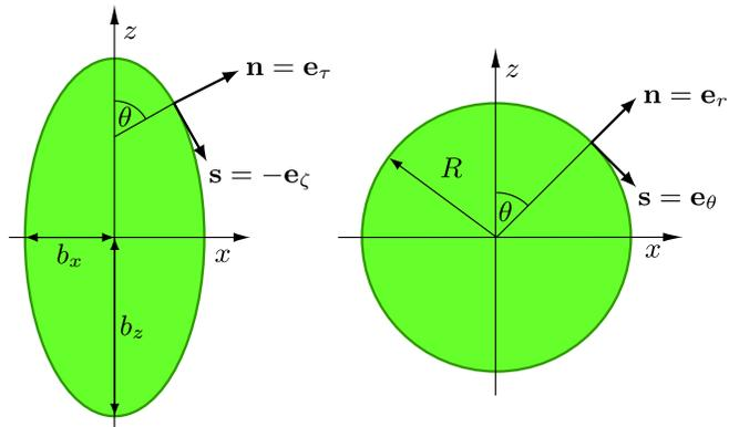
FIG. 1. Illustration of normal and tangent vectors of a spheroidal (left) and spherical (right) squirmer. Self-propulsion along the body-fixed orientation vector  $\mathbf{e}$ , here  $\mathbf{e} = (0, 0, 1)^T$ , is achieved by an axisymmetric prescribed surface velocity in the direction of the tangent vector  $\mathbf{s}$  [43].
