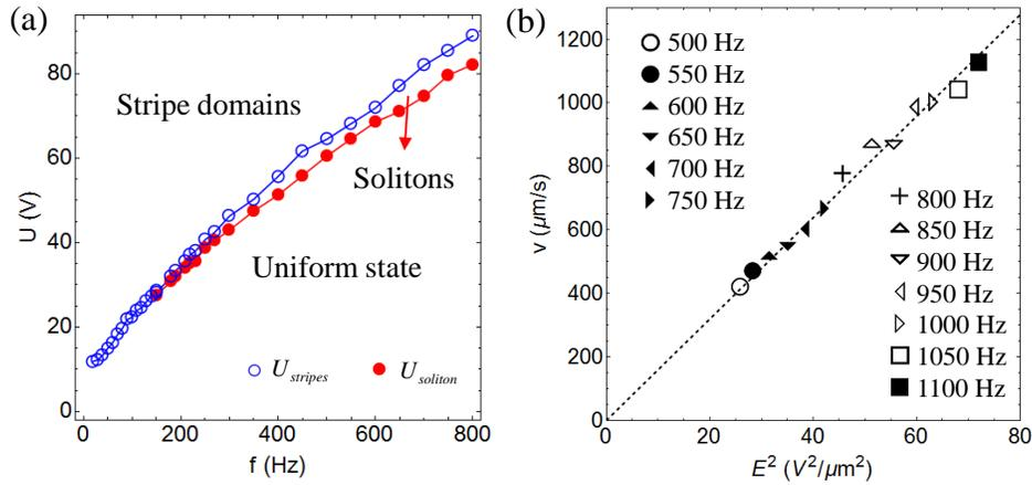
**Fig. 2 Soliton properties as a function of the applied field.** (a) Frequency dependencies of  $U_{soliton}$  and  $U_{stripes}$  ( $8.0\ \mu\text{m}$ ,  $45^\circ\text{C}$ ). (b) Velocity of solitons vs. square of the electric field ( $7.8\ \mu\text{m}$ ,  $50^\circ\text{C}$ ); the applied field corresponds to the frequencies specified in the legend.
