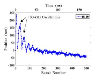
FIG. 4: Vertical centroid oscillations shown at rf BPM location B120 for 500 b, 500 pC/b, and V101=+1A. The 100-kHz oscillation decays noticeably in the first 200 b, and a centroid slew continues to the end of the macropulse.
