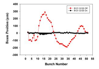
Figure 8: Comparison of the 50-bunch centroid oscillations at B121 located after the Q118-120 quadrupole triplet with V101= -1A. The downstream B121 location shows the oscillation amplitude was much reduced to about 30  $\mu$ m in the Q120 powered ON case. The beam actually appears to be over focused since the deflection phase is the opposite of the Q120 OFF case as confirmed in Fig. 9.
