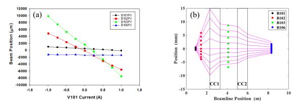
FIG. 3: (a) Macropulse-averaged vertical beam positions tracked with rf BPMs before, between, and after the two capture cavities versus the V101 corrector settings. (b) Beam positions relative to the 0-A case as a function of BPM position for a sequence of V101 corrector settings.
