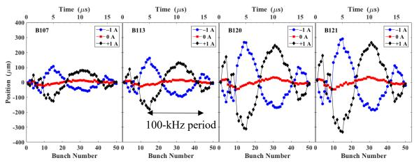
FIG. 5: Centroid vertical oscillations at 100 kHz shown at rf BPM locations B107, B113, B120, and B121 downstream of CC2. The three curves are for corrector currents at V101=-1, 0, +1 A, respectively. A strong correlation of sub-macropulse beam motion with V101 current was seen, consistent with excited HOMs as in Fig. 2.
