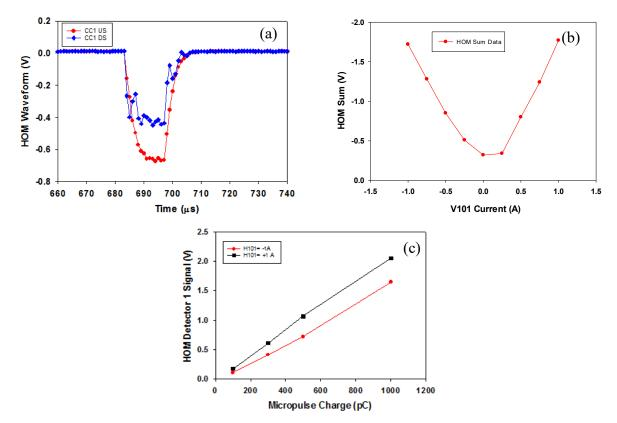
FIG. 2: a) Examples of the CC1 upstream and downstream HOM detector waveforms for 50 b at V101=1 A b) Measured sums of the 4 HOM detector signal peak values as a function of the vertical corrector current (V101) for 500 pC/b and c) plot of the near linear dependence on Q of CC1 HOM detector 1 for H101= -1 and +1 A from the reference current.
