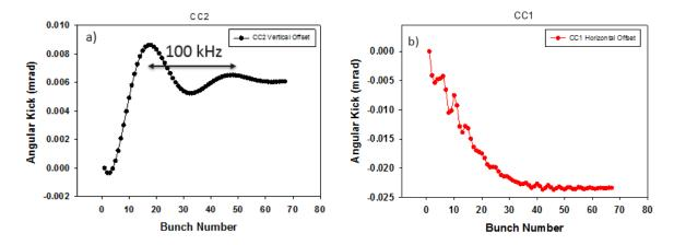
Figure 10: Calculational results for 500 pC/b and a 5-mm beam offset entering CC1 and CC2 a) the vertical steering and vertical oscillation for CC2 (M14) generated dipole HOMs and b) the horizontal steering and horizontal position oscillations for CC1 (M7 and M30) generated dipole HOMs.
