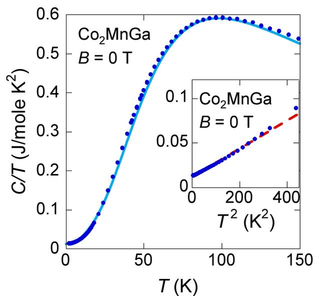
**Figure S3 | Specific heat for  $\text{Co}_2\text{MnGa}$  at low temperatures.** Temperature dependence of the specific heat divided by  $T$ ,  $C/T$ , for  $\text{Co}_2\text{MnGa}$  measured at  $B = 0$  T. The solid curve indicates the fit to the Debye formula. The inset shows the plot of  $C/T$  vs.  $T^2$  below  $T \sim 20$  K. The broken line indicates a linear fit.
