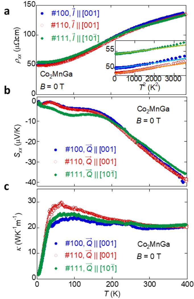
**Figure S2 | Electric and thermal transport properties for  $\text{Co}_2\text{MnGa}$ .** a-c, Temperature dependence of the longitudinal electric resistivity (a), Seebeck effect (b) and thermal conductivity  $\kappa$  (c) measured at  $B = 0$  with different heat current ( $\vec{Q}$ ) directions. Inset of a shows  $T^2$  dependence of the longitudinal electric resistivity  $\rho_{xx}$ . The solid lines indicate linear fits.
