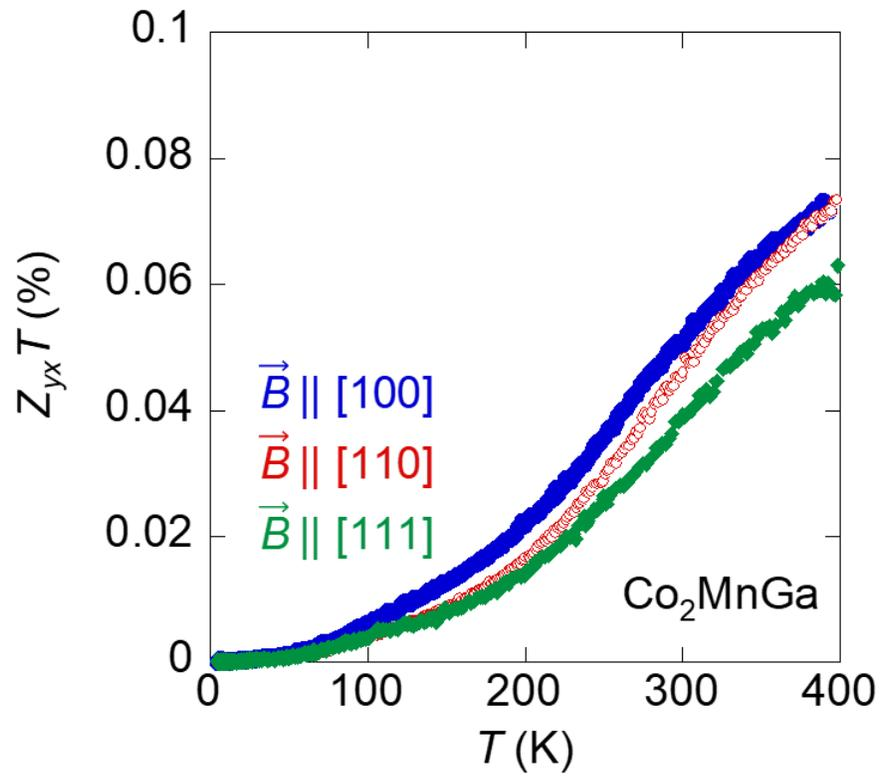
**Figure S7| Figure of merit for the Nernst effect of  $\text{Co}_2\text{MnGa}$ .** Temperature dependence of the figure of merit  $Z_{yx}T$  for the Nernst effect measured in the magnetic field along [100] (blue), [110] (red), and [111] (green) for  $\text{Co}_2\text{MnGa}$ .
