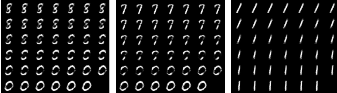
Figure 8: First and the last image of each panel show two k -means centroids in code space obtained on the MNIST dataset. Additional numbers are generated by “walking” on interpolated points between the two centroids.
