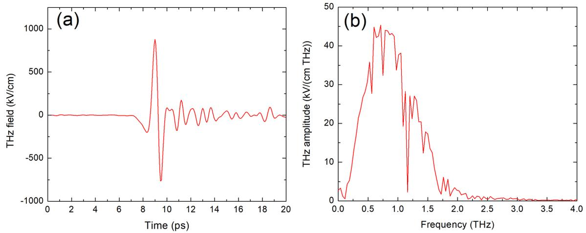
**Figure S1 Terahertz pump waveform:** **a** Electro-optic sampling signal of terahertz (THz) pump at sample location measured in-situ by electro-optic sampling in a 50  $\mu\text{m}$  thick (110) GaP crystal. **b** Amplitude spectrum of the THz waveform in **a**. Intensity adjusted with wiregrid polarizers (Infraspecs P01) without changing THz waveform.
