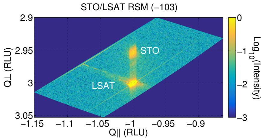
**Figure S3: Reciprocal space map of the sample before annealing.** Static reciprocal space map collected on a similar sample prior to annealing about the  $(-1\ 0\ 3)$  reciprocal lattice point using a  $\text{Cu } \alpha$  source. The separation between the film and substrate peaks along the cross-plane direction shows there is a difference in lattice parameter, whereas there is clear indication that in-plane the film and substrate are lattice matched to the LSAT unit cell.
