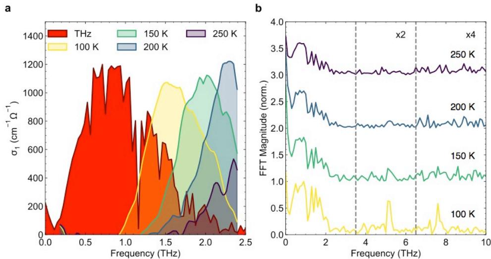
**Figure 3: Temperature dependence of sample response.** *a*, Optical conductivity data measured by THz ellipsometry show the temperature dependence of the soft phonon mode. Only at the lowest temperatures is there significant overlap with the THz pump spectrum (red area, normalized units) to drive the soft mode into the nonlinear regime. *b*, Fourier transform of trXRD signal showing transfer to high frequency modes at the corresponding temperatures in *a*.
