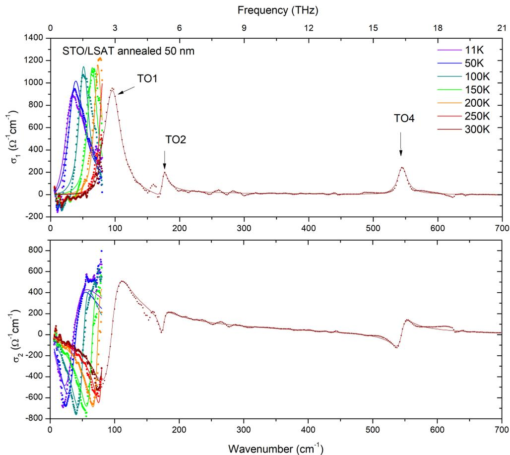
**Figure S4: Optical conductivity of the annealed sample.** We show additional ellipsometry measurements on our sample incorporating extra temperature points at low and high temperature. The extended frequency range at 300K shows the  $\text{TO}_2$  and  $\text{TO}_4$  phonon modes. Data from Fig. 3a are also included for comparison.
