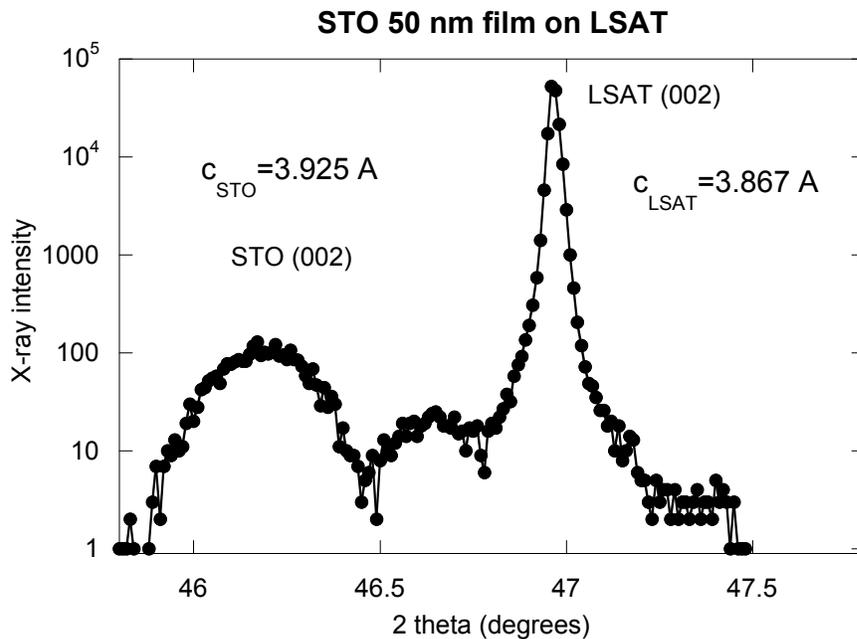
**Figure S2: Two-Theta scan of sample before annealing.** Static x-ray diffraction pattern along sample normal. The low-angle peak corresponds to the STO film and the sharp peak at higher angle is the LSAT substrate. We observe clear splitting along the cross-plane direction between the substrate and the film. These measurements were taken before the sample was annealed.
